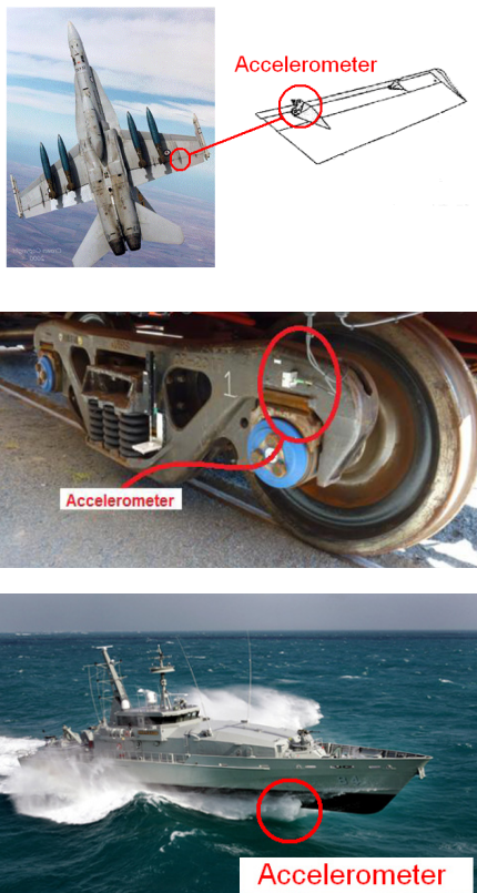
Figure 2. Accelerometer locations. Upper – in-board aileron hinge of a fast jet. Centre – bogey of a heavy-haul rail-car. Lower – bow of a boat.
