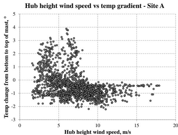
**Figure 11.** Temperature gradients with hub height wind speed at Site A
