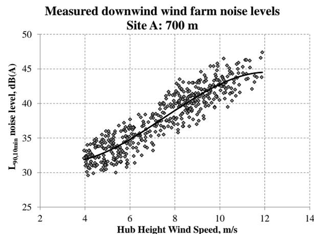
Figure 6. Measured downwind wind farm noise levels at location 700 m from Site A
