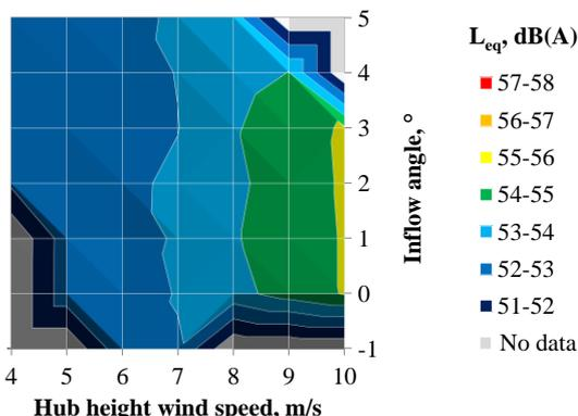
**Figure 16.** Average A-weighted SPL at Site B turbine with hub height wind speed and inflow angle
