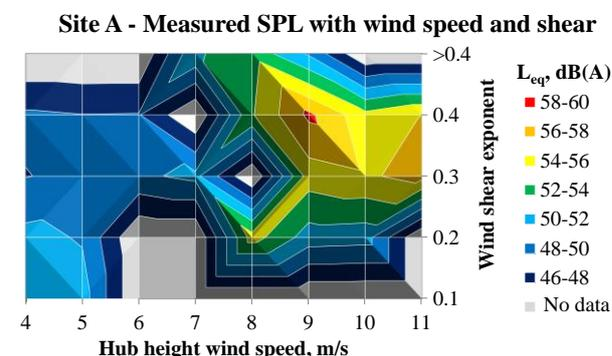
Figure 1. Average A-weighted SPL at Site A turbine with hub height wind speed and wind shear
