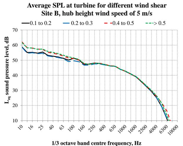
Figure 4. Average SPL at Site B turbine for different wind shear values and hub height wind speed of 5 m/s
