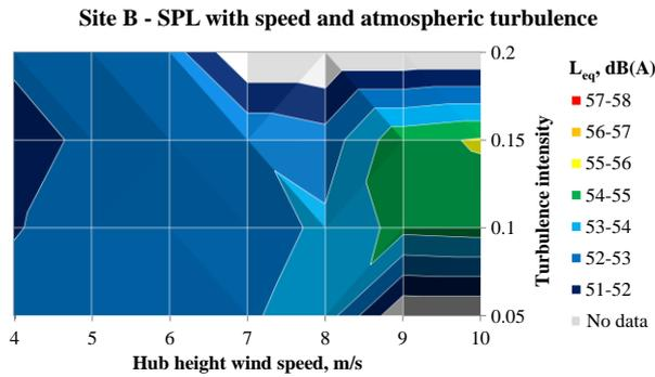
**Figure 13.** Average A-weighted SPL at Site B turbine with hub height wind speed and atmospheric turbulence intensity
