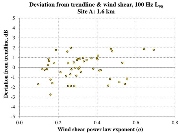
**Figure 8.** Deviation in measured  $L_{90}$  noise level in 100 Hz one-third octave band from trendline with wind shear at location 1600 m from Site A
