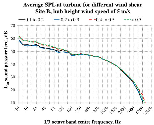
Figure 4. Average SPL at Site B turbine for different wind shear values and hub height wind speed of 5 m/s
