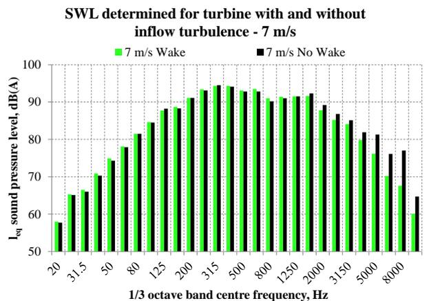
**Figure 15.** Calculated sound power level of turbine for 10 m height wind speeds under wake and non-wake conditions
