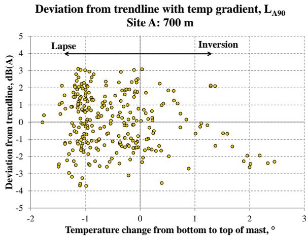
**Figure 10.** Deviation in measured noise level from trendline with temperature gradient at location 700 m from Site A
