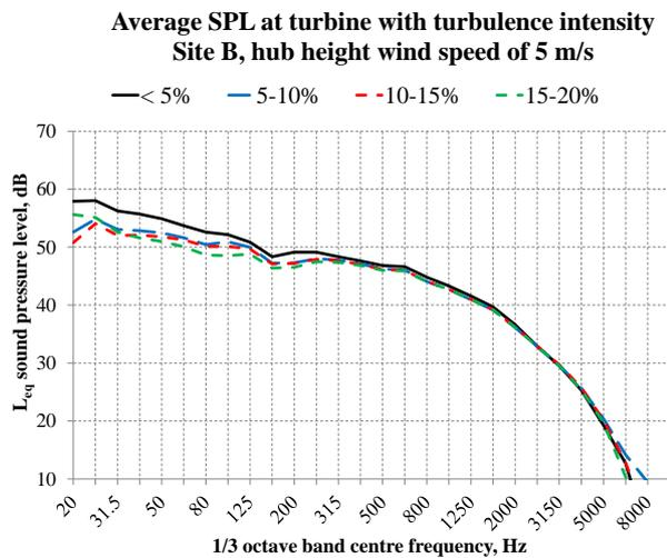
**Figure 14.** Average SPL at Site B turbine for different turbulence intensity at a hub height wind speed of 5 m/s
