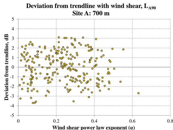
Figure 7. Deviation in measured  $L_{A90}$  noise level from trendline with wind shear at location 700 m from Site A
