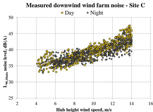
Figure 5. Measured downwind wind farm noise levels at 1.5 km from Site C for day and night periods
