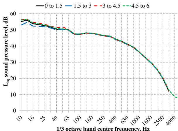
**Figure 17.** Average SPL at Site B turbine for inflow angles at a hub height wind speed of 5 m/s
