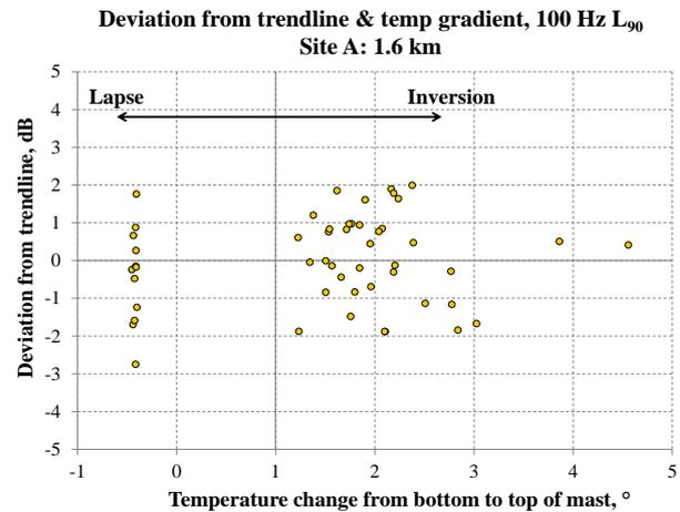
**Figure 12.** Deviation in measured  $L_{90}$  noise level in 100 Hz one-third octave band from trendline with temperature gradient at location 1600 m from Site A
