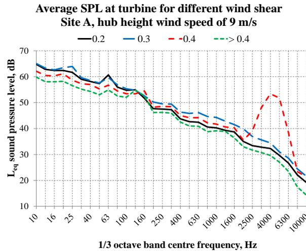
Figure 2. Average SPL at Site A turbine for different wind shear values and hub height wind speed of 9 m/s
