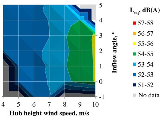
**Figure 16.** Average A-weighted SPL at Site B turbine with hub height wind speed and inflow angle
