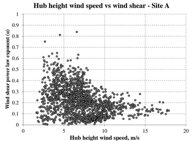
**Figure 9.** Wind shear values with hub height wind speed at Site A
