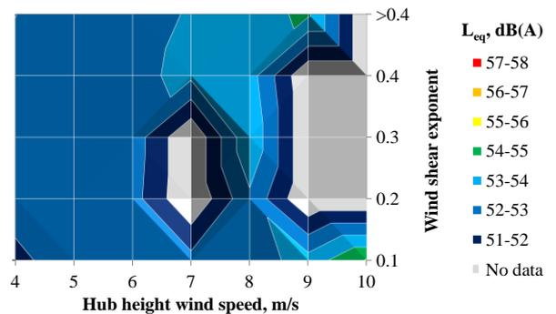
Figure 3. Average A-weighted SPL at Site B turbine with hub height wind speed and wind shear
