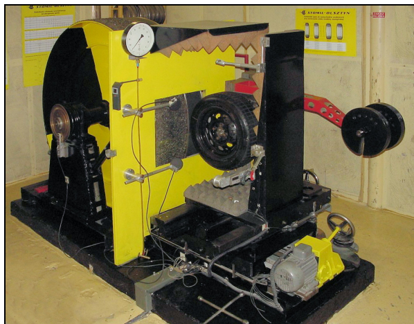
Figure 3. The drum facility at TUG used for testing noise emission and rolling resistance the PERS material. The drum diameter is 1.7 m.
