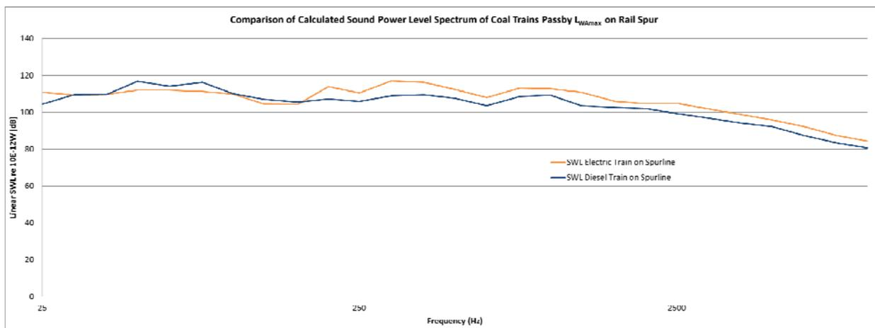
Figure 5. Comparison of Calculated Spectrums of  $L_{WAmax}$  SWL for Coal Train Passby on Rail Spur (25Hz to 10kHz)
