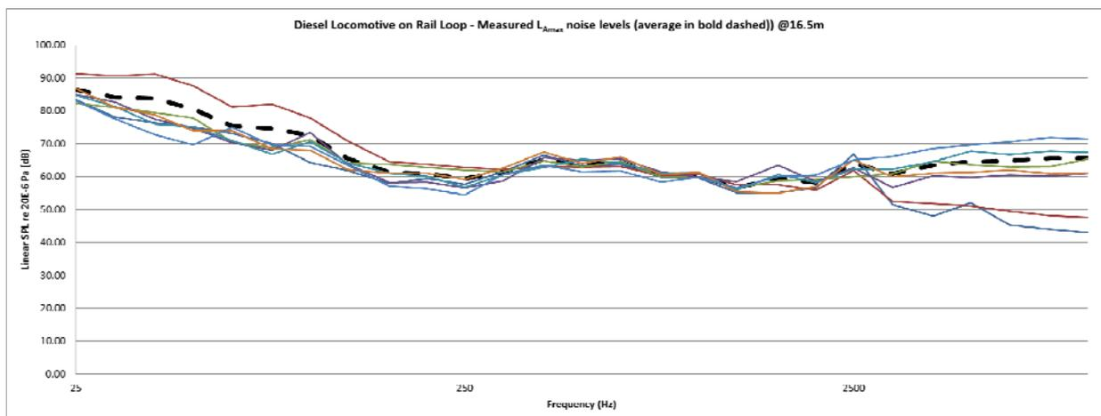
Comparisons of the calculated sound power levels based on the measured levels from passing electric and diesel powered coal trains are shown in Figures 5 to 8. Figures 5 and 6 show the comparison of maximum and average sound power levels for coal train passbys on the spur line for electric and diesel trains, while Figures 7 and 8 show the comparison of maxi-
