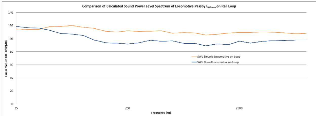
Figure 7. Comparison of Calculated Spectrums of  $L_{WAmax}$  SWL for Locomotive Passby on Rail Loop (25Hz to 10kHz)
