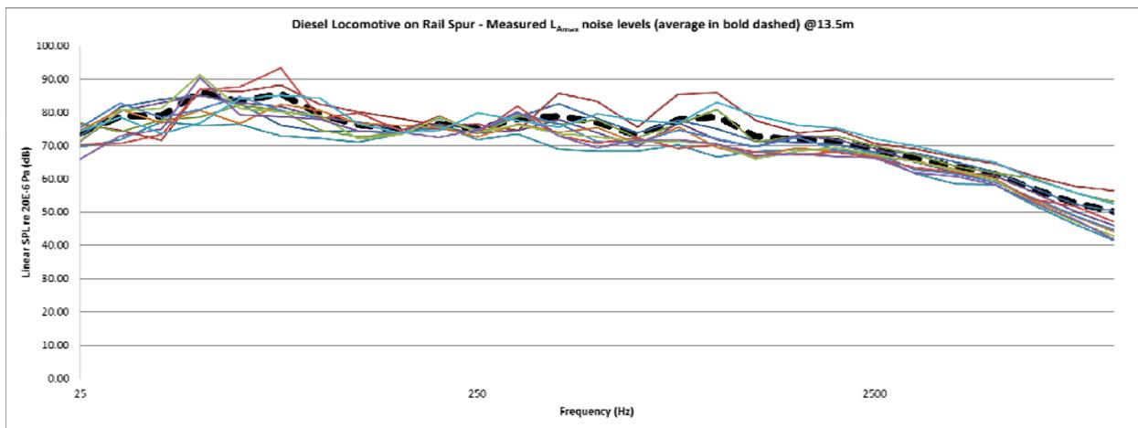
**Figure 2.** Measured Spectrum of  $L_{Amax}$  SPL for Diesel driven trains on Rail Spur @13.5m (25Hz to 10kHz)
