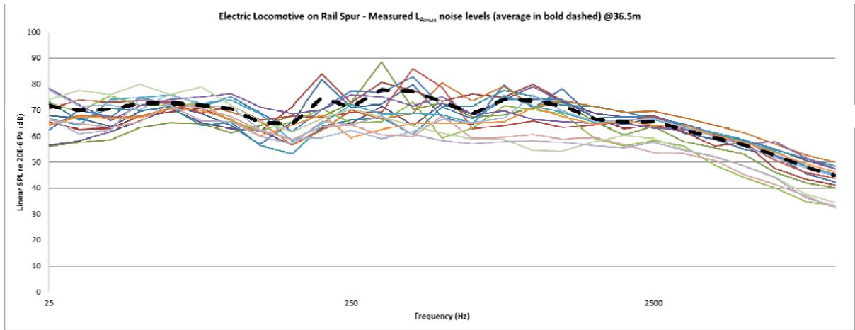
**Figure 1.** Measured Spectrum of  $L_{Amax}$  SPL for Electric driven trains on Rail Spur @36.5m (25Hz to 10kHz)
