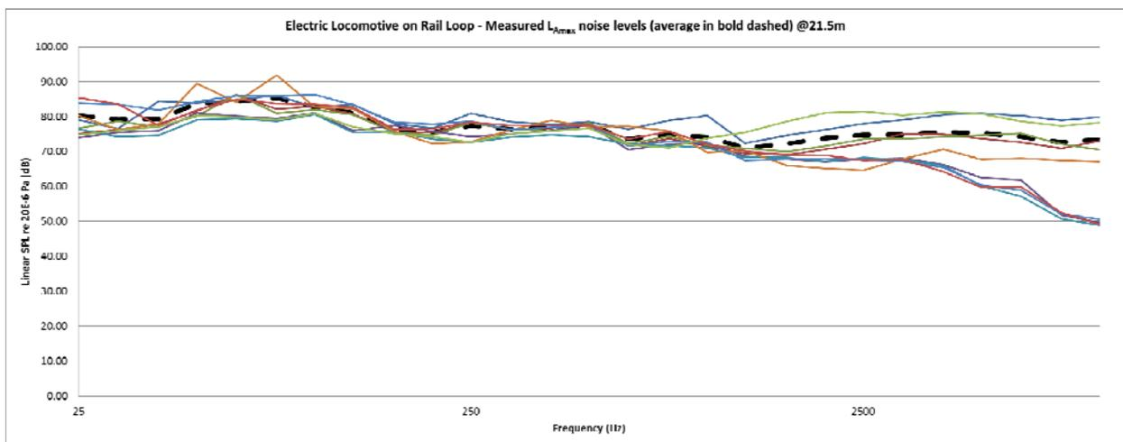
**Figure 3.** Measured Spectrum of  $L_{Amax}$  SPL for Electric Locomotives on Rail Loop @21.5m (25Hz to 10kHz)
