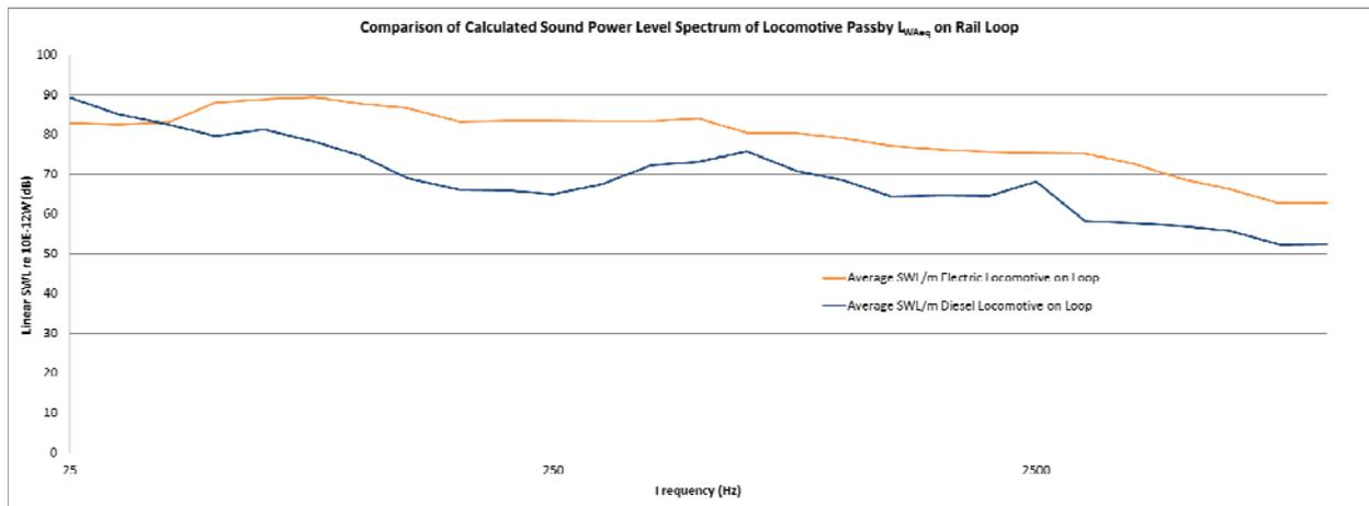
Figure 8. Comparison of Calculated Spectrums of  $L_{WAeq}$  SWL/m for for Locomotive Passby on Rail Loop (25Hz to 10kHz)
