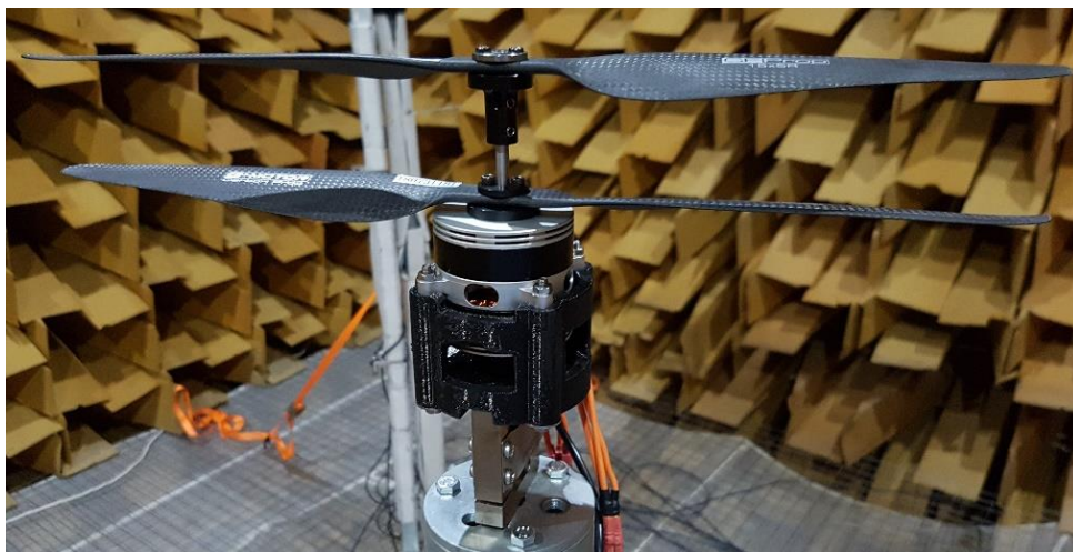
Figure 1. Contra-rotating motor with 15" propellers spaced 48 mm apart. The motor was mounted on a load cell in the University of Auckland's anechoic chamber.
