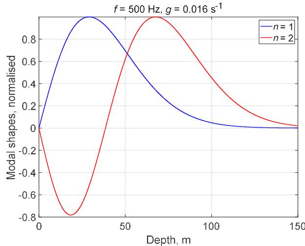
Figure 1: Vertical profiles of the first two modes in the medium under consideration;  $f$ ,  $g$  and  $n$  are the acoustic frequency, the sound speed gradient, and the mode number respectively
