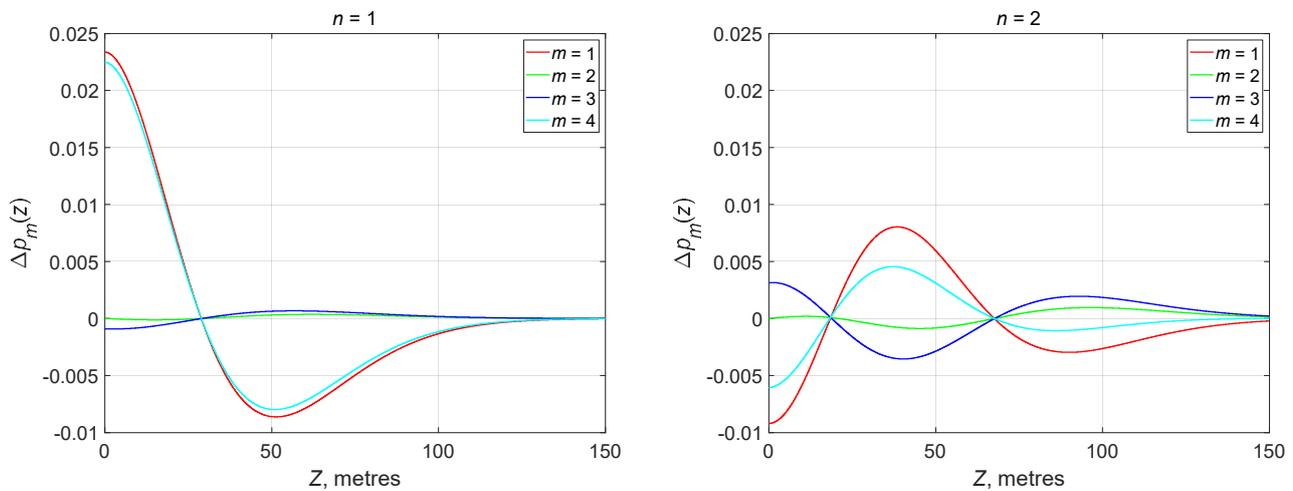
Figure 2: Differences between normalised vertical pressure profiles determined by Eq. (15) for the first and second normal modes
