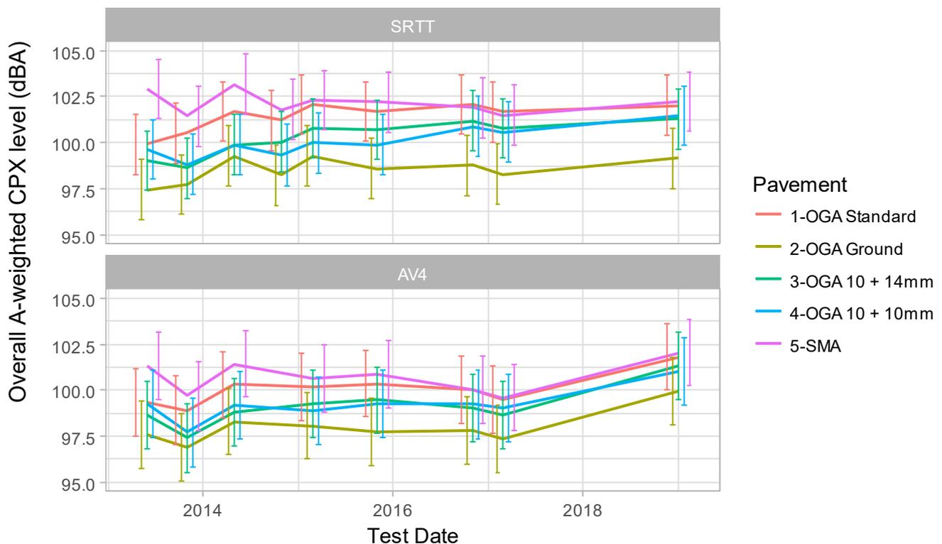
Figure 5: Long term performance (Overall A-weighted CPX level, dBA) over five years
