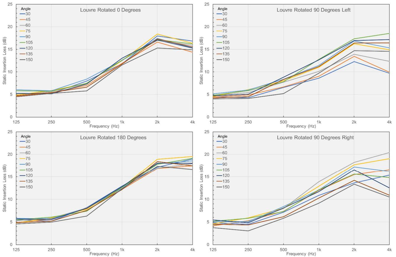
Figure 8: Static insertion loss for the louvre in the external wall of the test facility at different orientations
