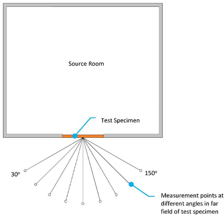
Figure 2: Configuration 1 for the static insertion loss testing
