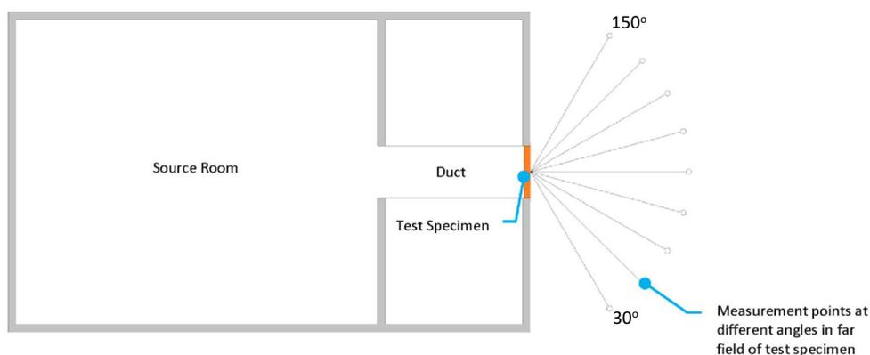
Figure 3: Configuration 2 for the static insertion loss testing
