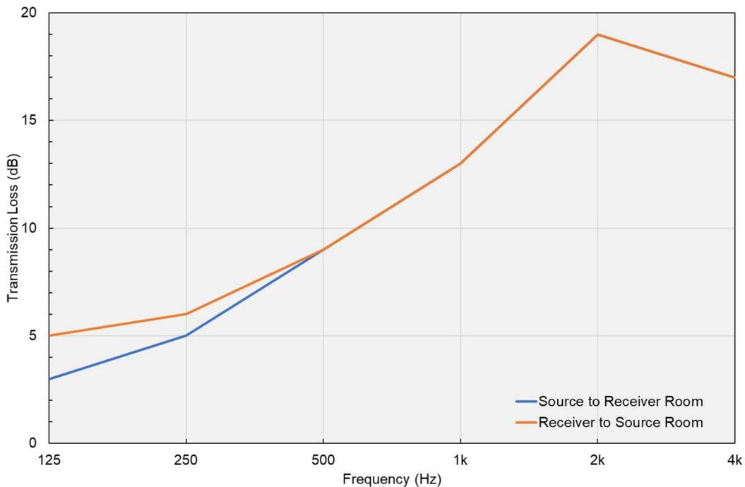
Figure 12: Transmission loss results
