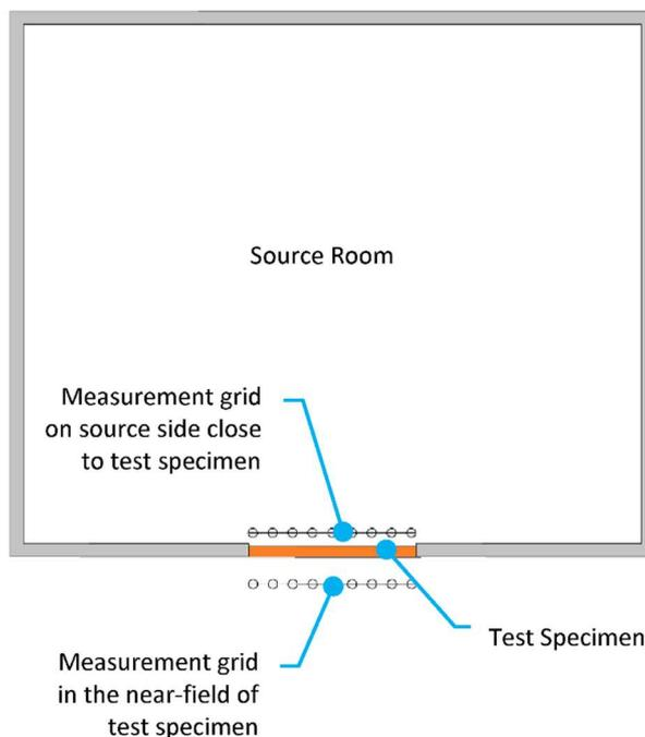
Figure 6: Measurement locations for the noise reduction testing
