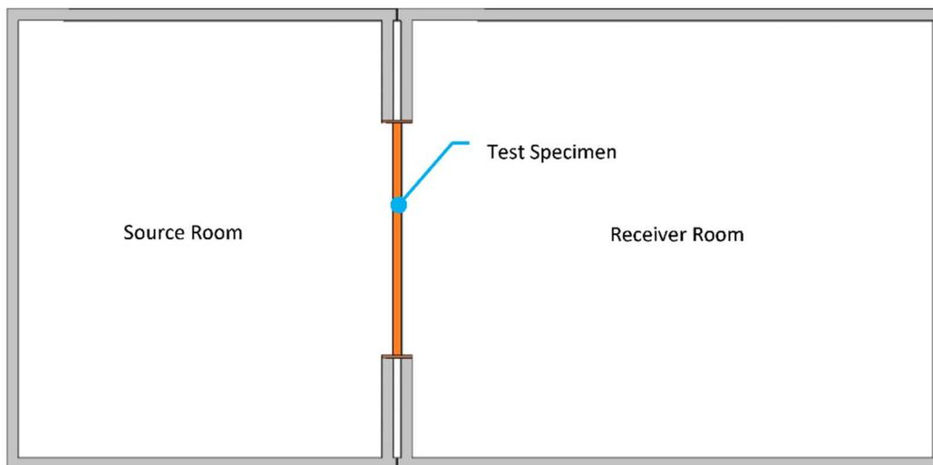
Figure 4: Schematic of the transmission loss suite
