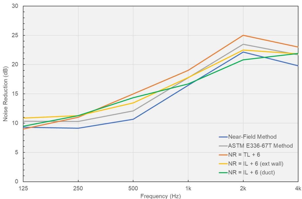
Figure 14: Comparison between ‘noise reduction’ results obtained using the different methods
