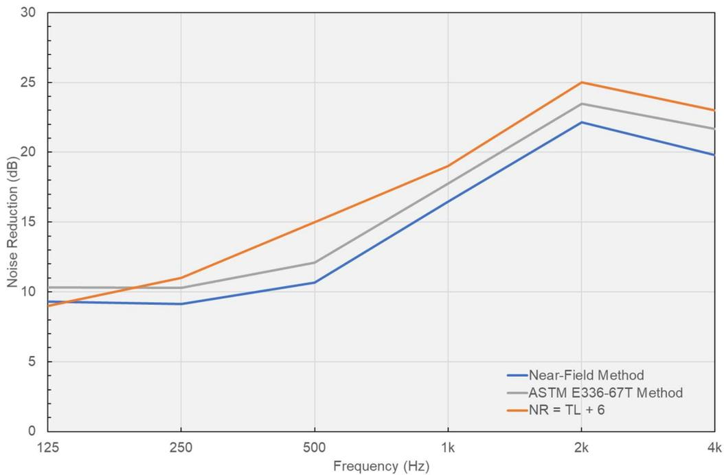
Figure 13: Measured and calculated noise reductions
