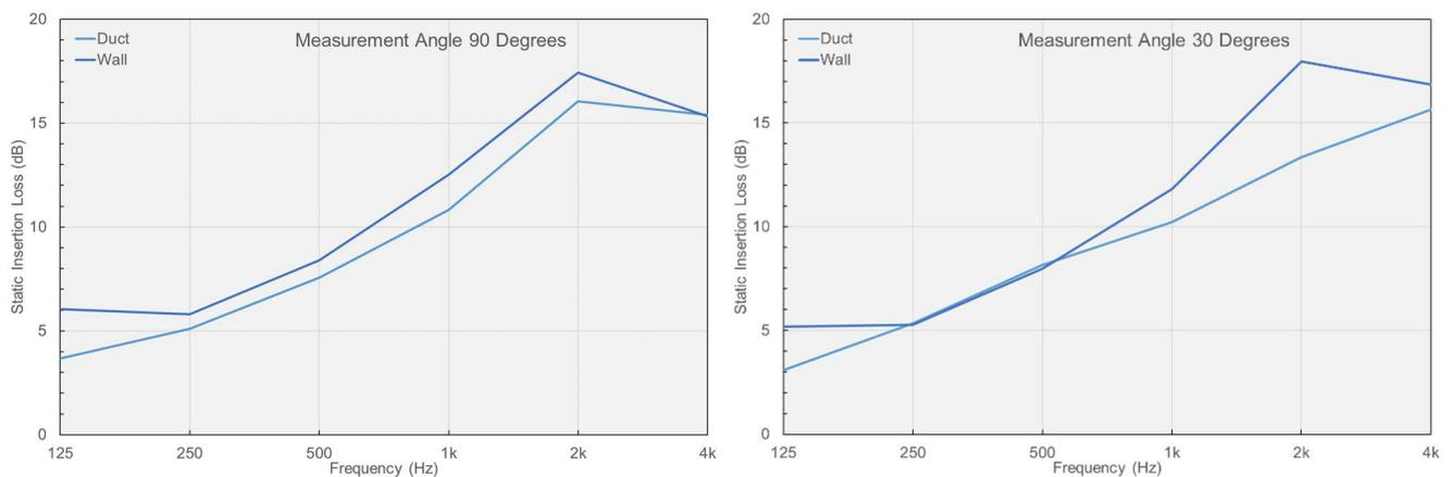
Figure 11: Comparison of static insertion loss measurement angle and directivity for louvre located in the external wall of the test facility and at the end of the duct
