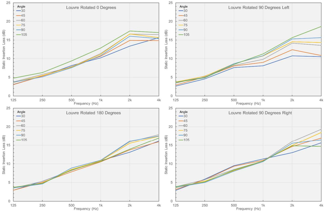
Figure 10: Static insertion loss with the louvre at the end of the duct for different orientations
