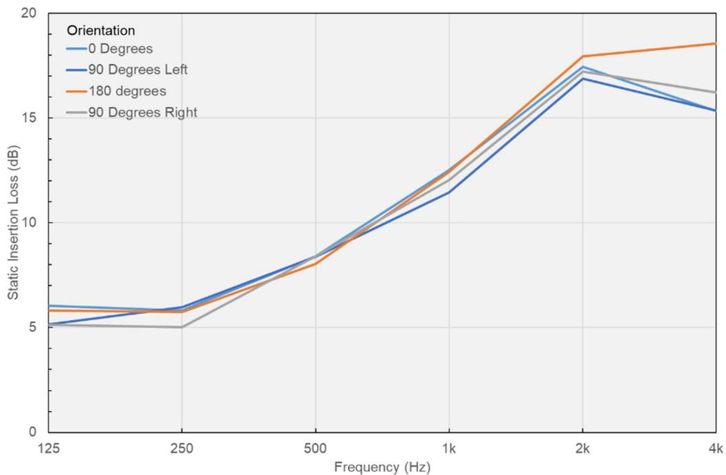
Figure 9: Static insertion loss at 90° with the louvre in the external wall of the test facility at different orientations
