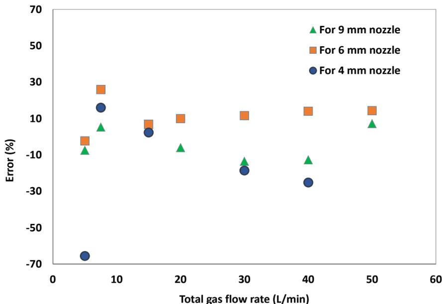
Figure 6 Relative differences between the predicted and measured gas flow rate
