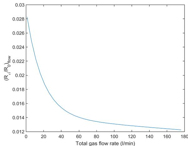
Figure 2 Correction  $C(Q)$  as function of gas flow rate
