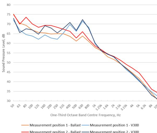
Figure 8 Ballast vs V300 spectra – Trip 3 (Comeng train)
