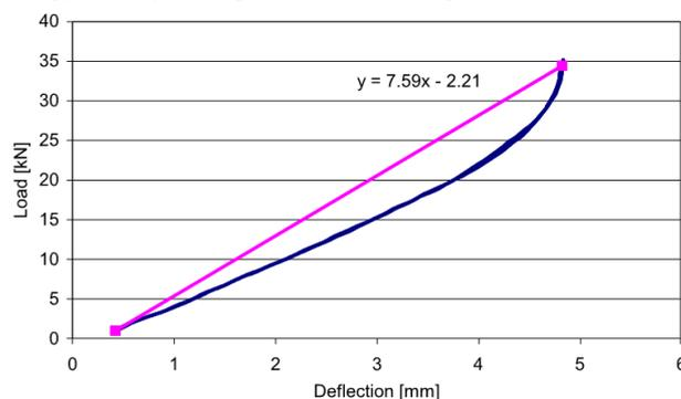
Figure 11 Dynamic load testing of rail pad system
