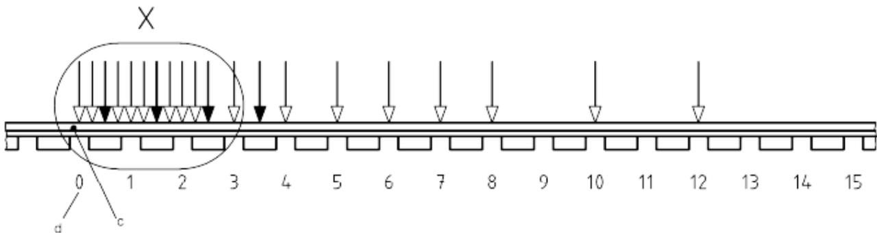
Figure 3 Diagram of impact locations for TDR measurements [from DIN EN 15461:2011-01]
