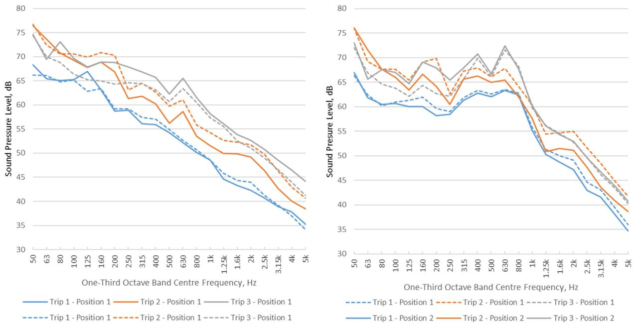
Figure 9 Ballast(left) vs V300(right) SPL spectra
