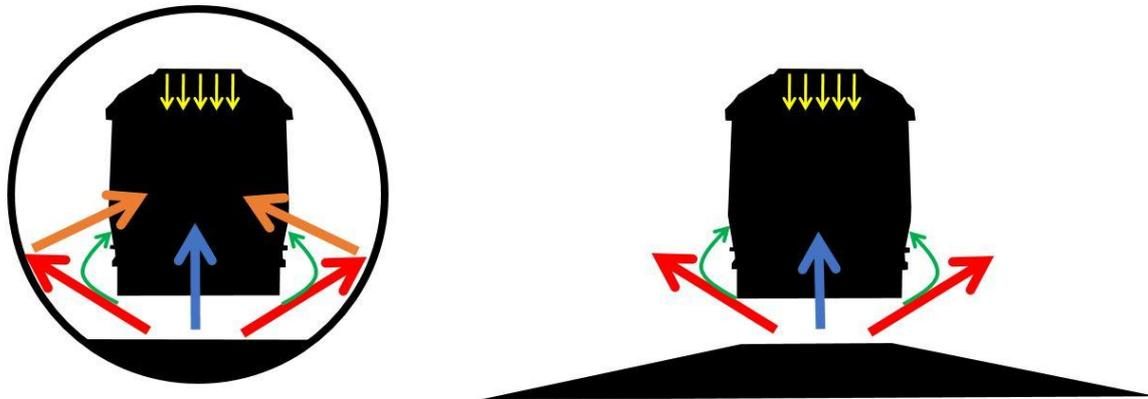
Figure 1 In-carriage noise emission paths, tunnelled railway, at-grade railway
