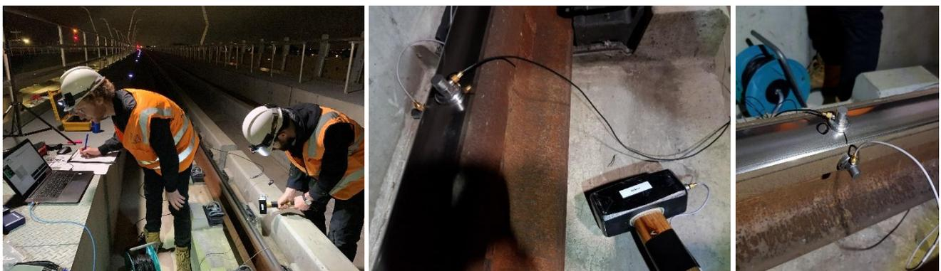
Figure 4 Track Decay Rate Measurements: On site personnel (left); accelerometers and instrumented hammer (centre); vertical and transverse accelerometers (right)
