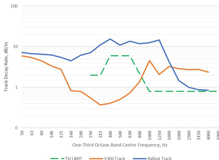
Figure 5 Track Decay Rate for V300 (on plinth) and Ballast (concrete sleeper) Trackforms
