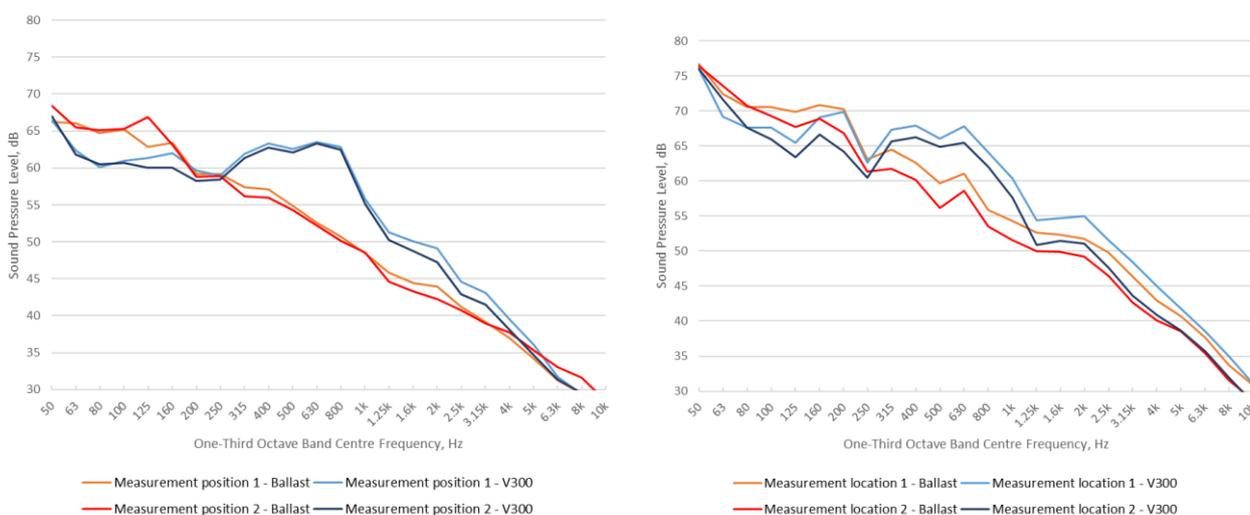
Figure 6 Ballast vs V300 spectra – Trip 1 (Siemens) & Figure 7 Ballast vs V300 spectra – Trip 2 (Comeng train)
