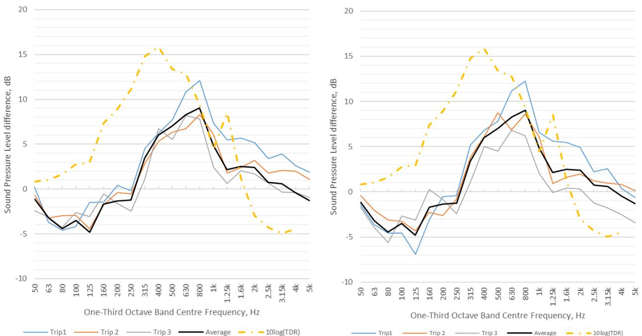
Figure 10 SPL differences – Ballast minus V300, position 1 (left) and position 2 (right)
