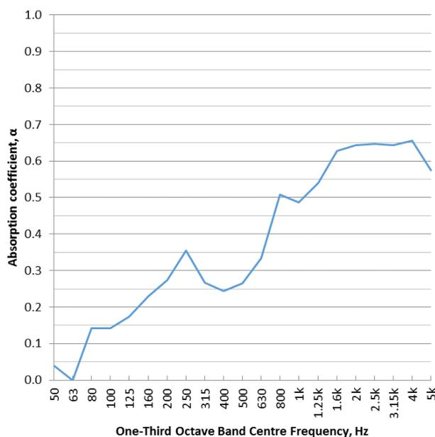
Figure 12 Absorption coefficient of 300mm thick ballast (Broadbent, 2009)
