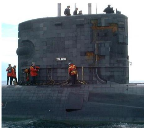
Figure 7 The UK submarine HMS Triumph. The outlines of anechoic tiles are visible as are areas where tiles are missing (Wikipedia, 2019).
