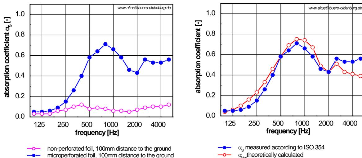
Figure 2: Measured result for sound absorption coefficient according to (ISO 354, 2003) for non-perforated and micro-perforated foil (left) and comparison between measurement and calculation.
