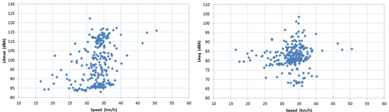
Figure 2:  $L_{Amax}$  (left) and  $L_{Aeq}$  (right) noise level at 1.2 m distance vs train speed, Site A
