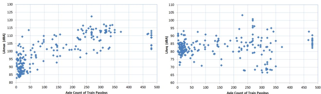
Figure 3:  $L_{Amax}$  (left) and  $L_{Aeq}$  (right) noise level at 1.2 m distance vs axle count of train passbys, Site A
