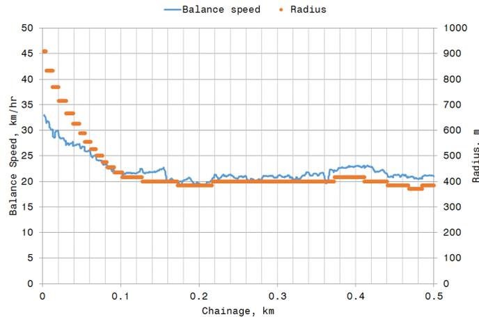
Figure 1: Estimated balance speed and curve radius versus chainage
