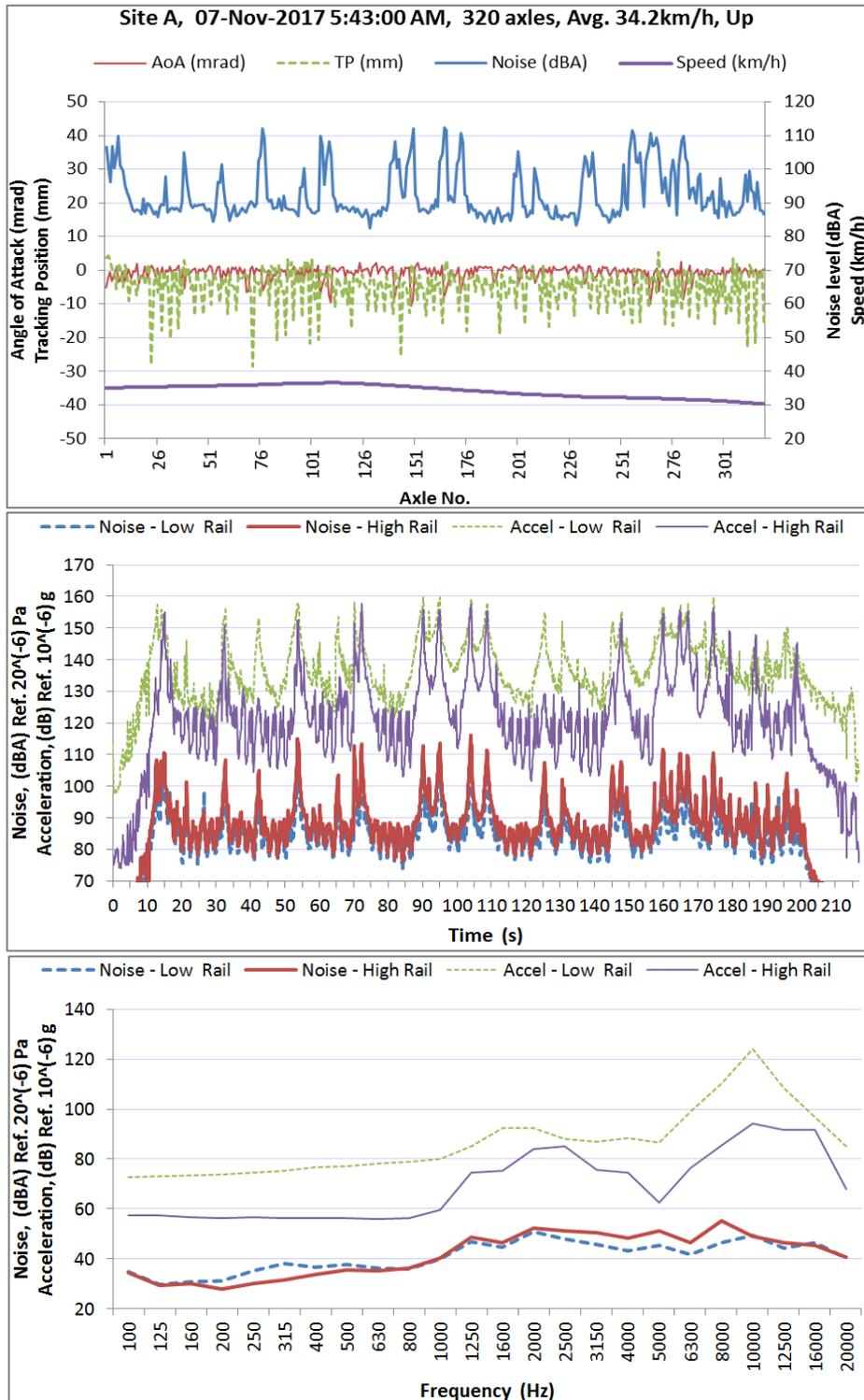
Figure 4: Example WNMS passby results, Site A: (top) overall AoA, TP, noise and vibration overall levels per axle; (middle) noise levels versus time; and (bottom) passby spectral sound pressure and acceleration levels.
