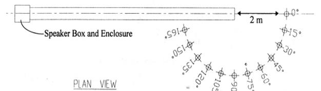
Figure 6: Measurement Schematic
