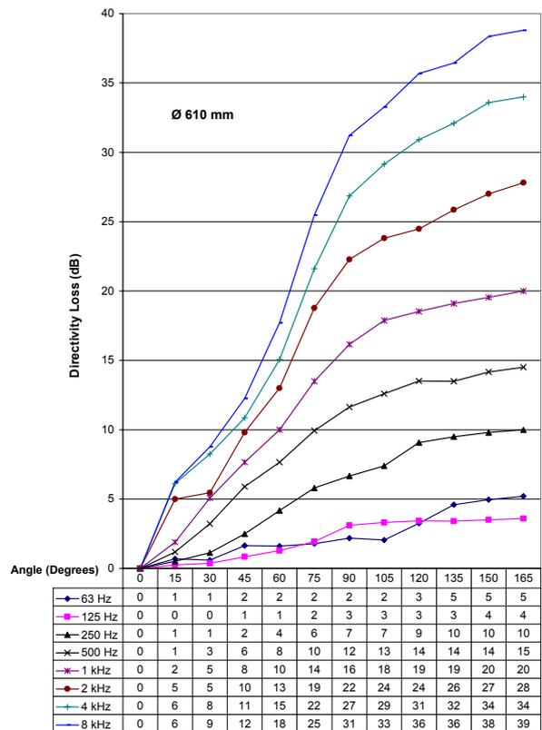
Figure 17: Ø 610 mm Duct Directivity Loss
