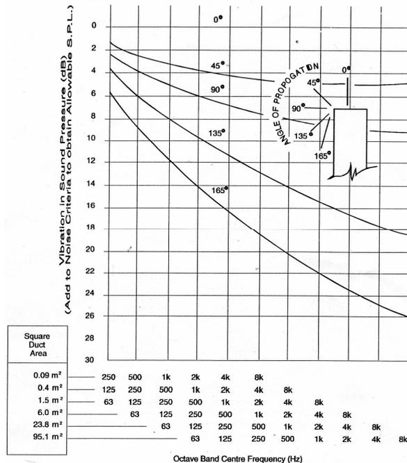
Figure 2: Directivity Loss in a Free Field (EPA Data Sheet 207-1,1994)
