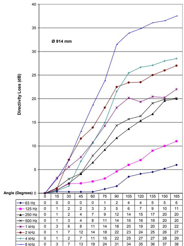
Figure 18: Ø 914 mm Duct Directivity Loss
