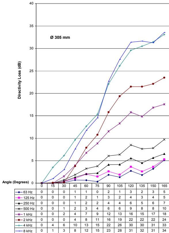
Figure 16: Ø 305 mm Duct Directivity Loss
