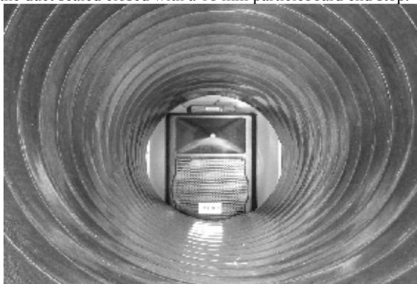
Figure 5: View of speaker inside duct
