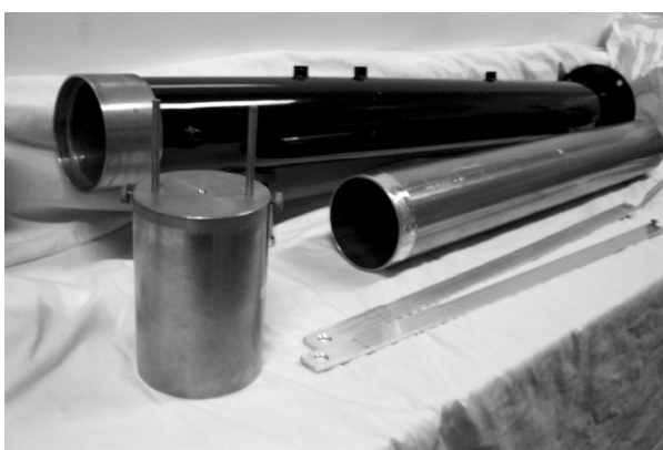
Figure 4. The modified standing wave tube (rear) for transfer function measurements of impedance, with the extension tube and retaining strap extensions in front.
