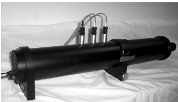
Figure 5. Impedance tube using the transfer function method.
