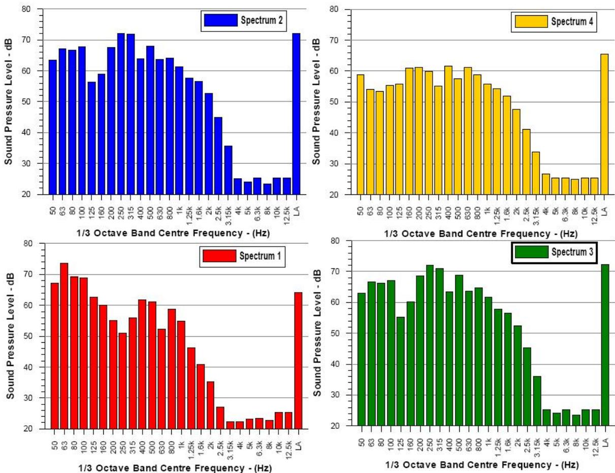
Figure 6. Helicopter Type 5 Spectrum Corresponding to Points in Figure 5 – Overflight 2000ft
