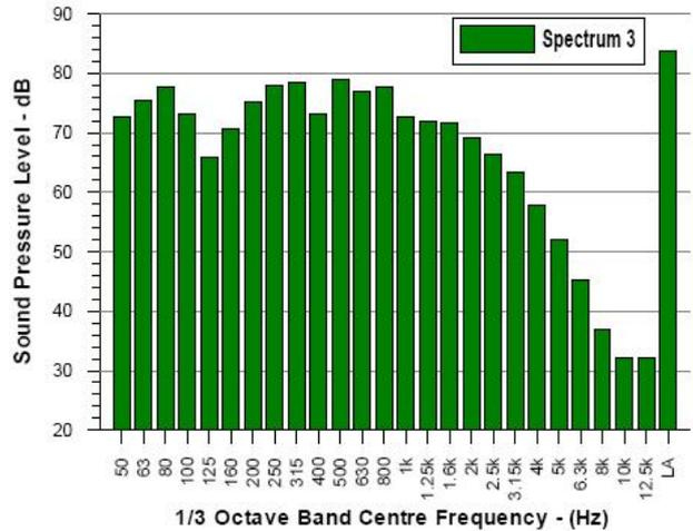
Figure 4. Helicopter type 5 Spectrum Corresponding to Points in Figure 3 – Overflight 500ft
