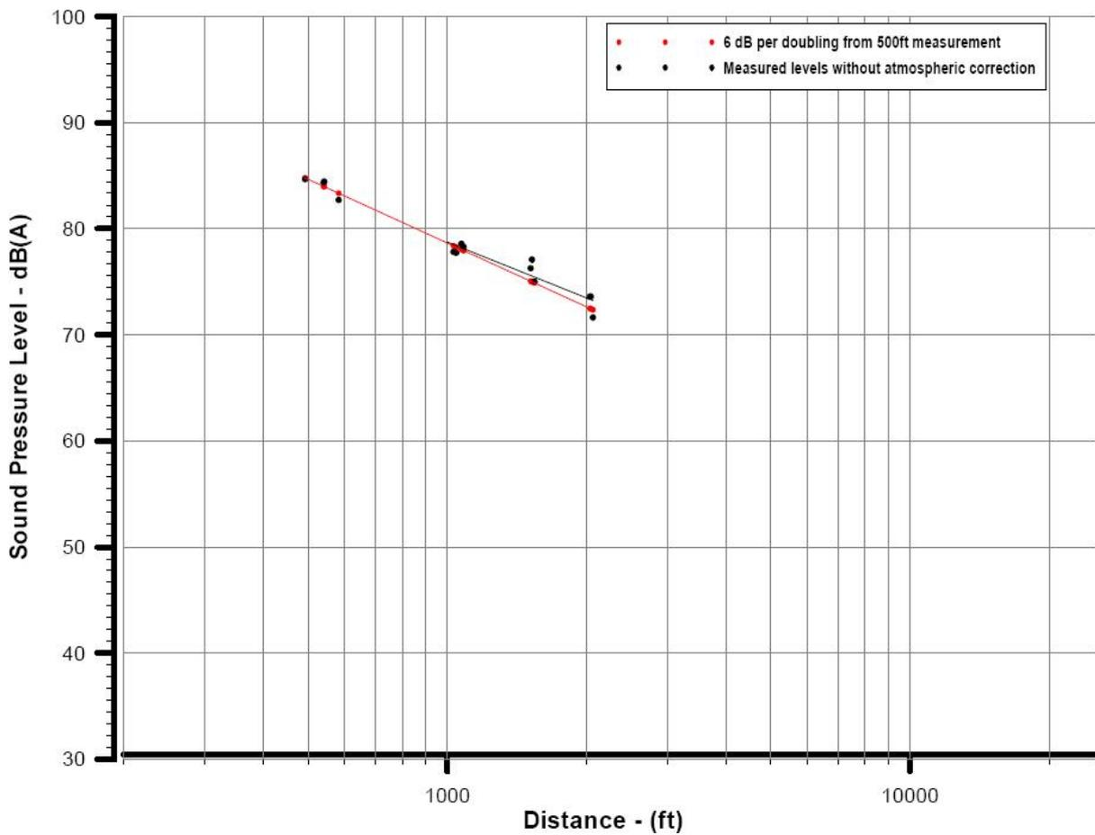
Figure 2. Helicopter Type 5 – Max Level without Atmospheric Correction
