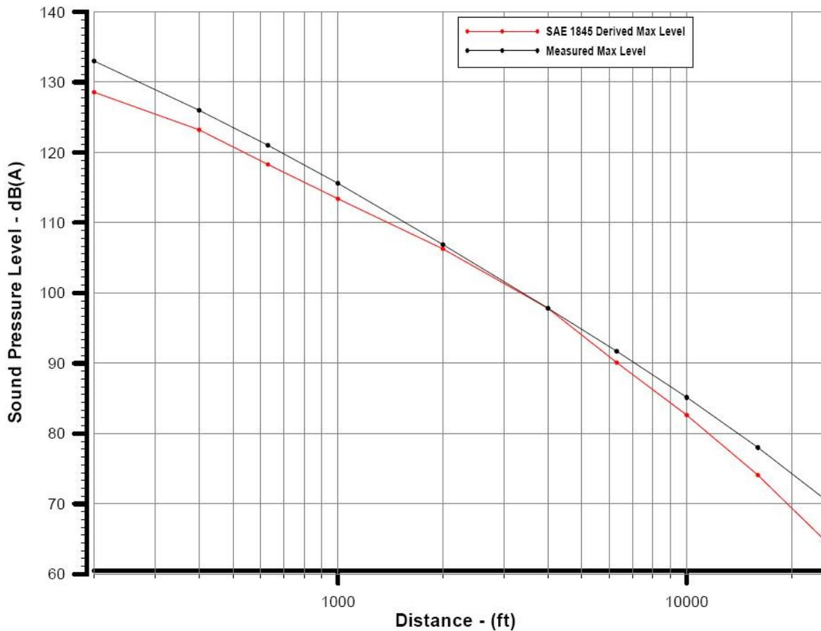
Figure 8. Twin Engine Military Jet – NPD Max Level
