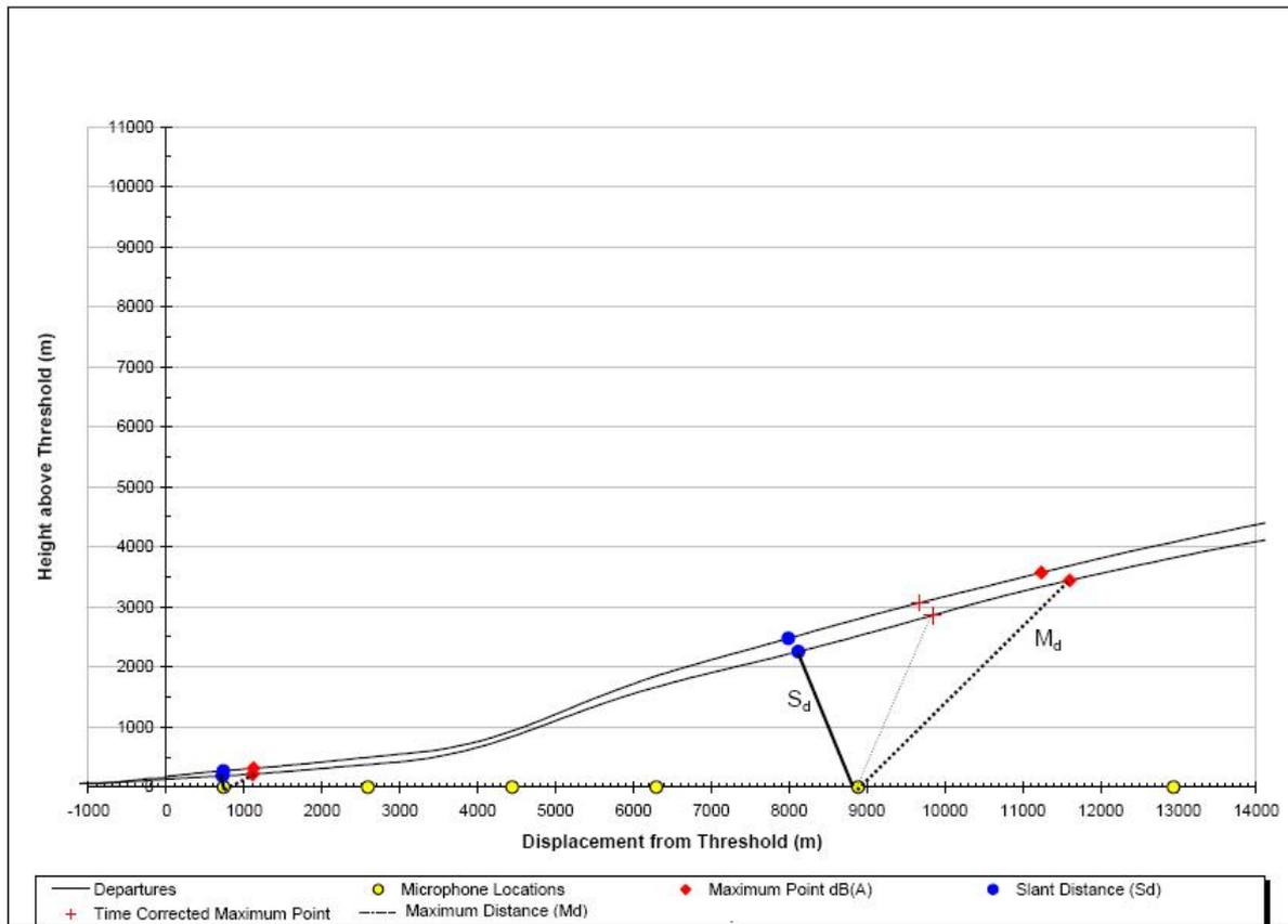
Figure 7. Twin Engine Military Jet – Departure with Afterburners Profile
