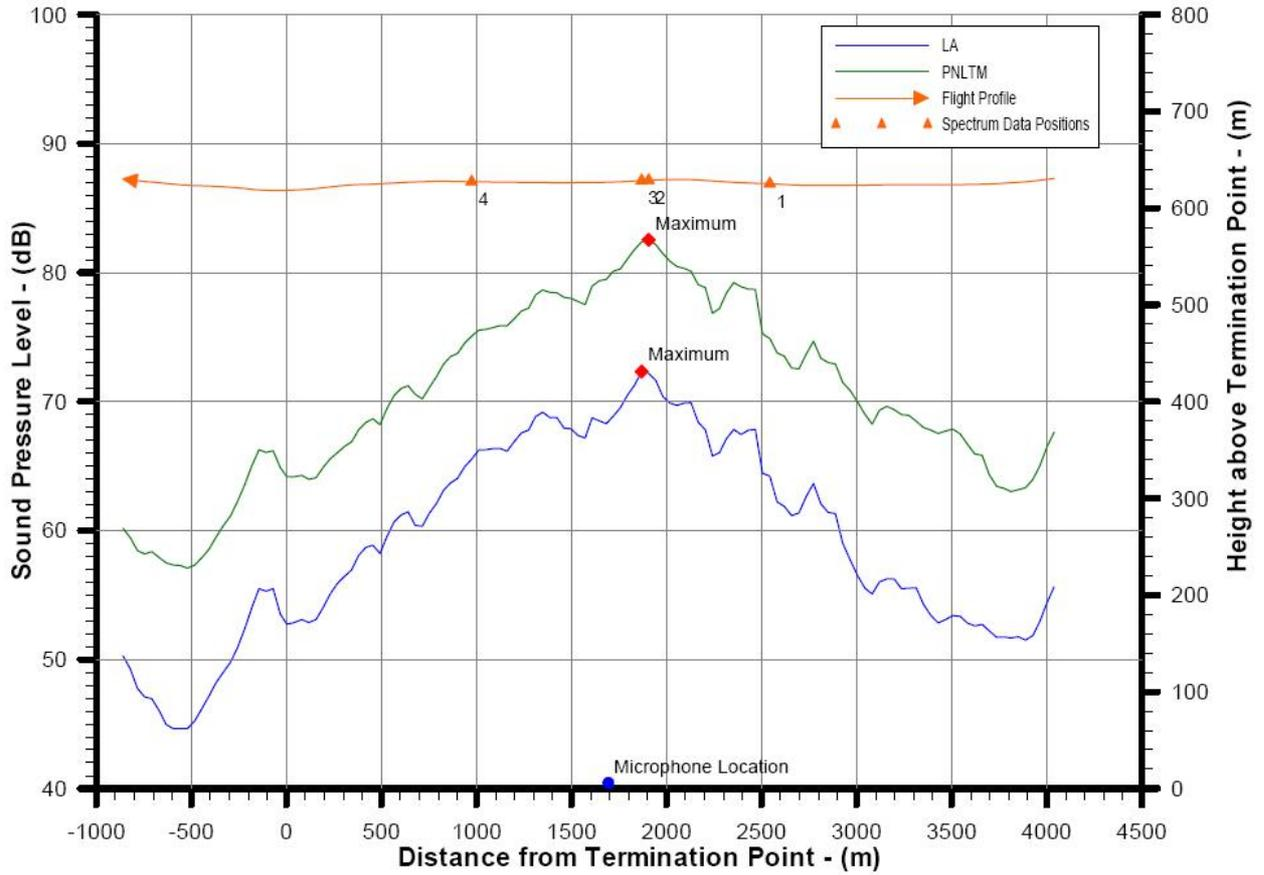
Figure 5. Helicopter Type 5 Flight Profile with dB(A) and PNLTM levels – Overflight 2000ft AGL
