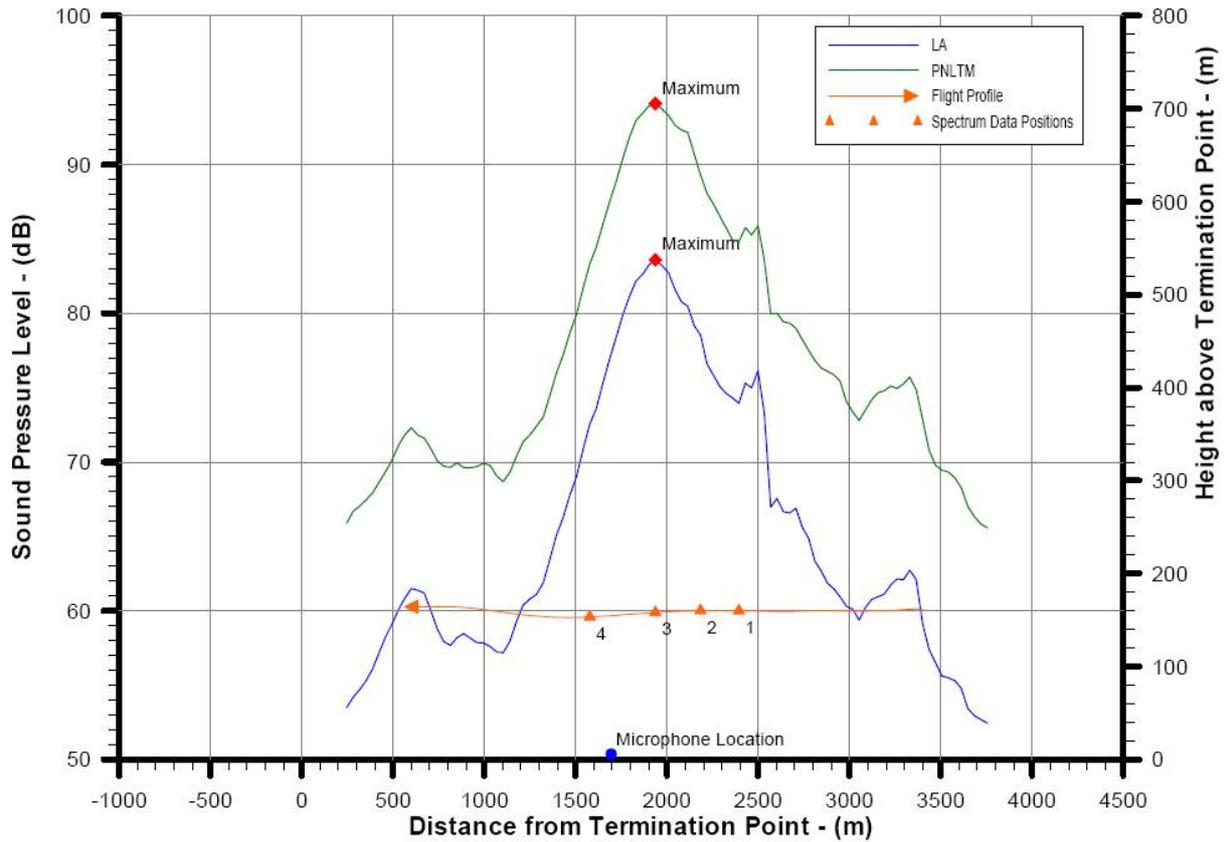
Figure 3. Helicopter Type 5 Flight Profile with dB(A) and PNLTM – Overflight 500 ft AGL
