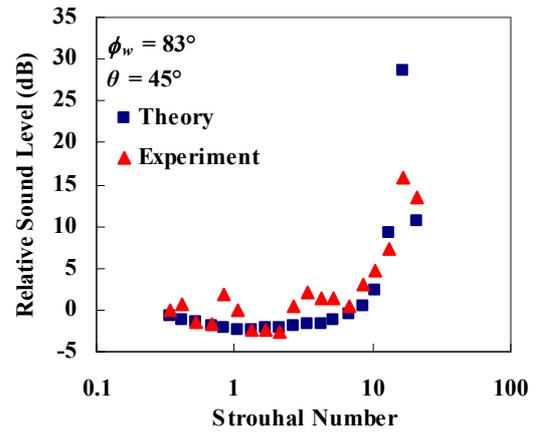
Figure 10. The sound level at  $45^\circ$  relative to that at  $0^\circ$  as a function of Strouhal number for 6 mm thick glass installed in the wall of a room.
