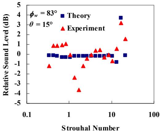
Figure 8. The sound level at  $15^\circ$  relative to that at  $0^\circ$  as a function of Strouhal number for 6 mm thick glass installed in the wall of a room.
