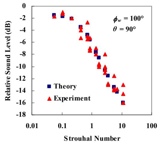
**Figure 17.** The sound level at 90° relative to that at 0° as a function of Strouhal number for an opening in the wall of a room.
