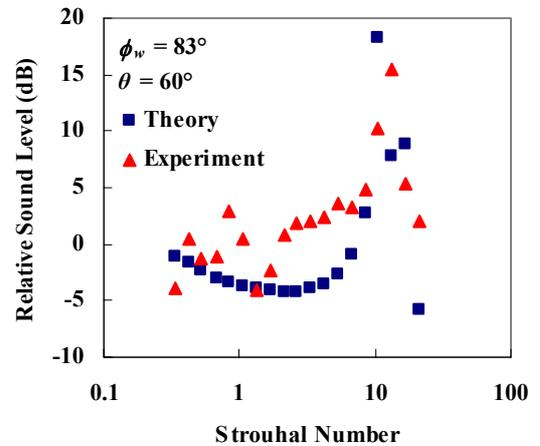
Figure 11. The sound level at  $60^\circ$  relative to that at  $0^\circ$  as a function of Strouhal number for 6 mm thick glass installed in the wall of a room.
