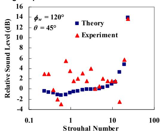
**Figure 2.** The sound level at  $45^\circ$  relative to that at  $0^\circ$  as a function of Strouhal number for 1 mm thick glass installed in the wall of a box.
