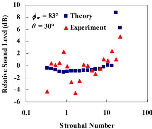
Figure 9. The sound level at  $30^\circ$  relative to that at  $0^\circ$  as a function of Strouhal number for 6 mm thick glass installed in the wall of a room.
