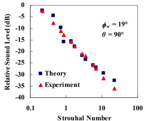
**Figure 22.** The sound level at 90° relative to that at 0° as a function of Strouhal number for an unbaffled duct end opening with a weighting angle of 19°.
