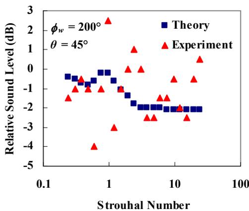
**Figure 14.** The sound level at 45° relative to that at 0° as a function of Strouhal number for opening in the wall of a box.
