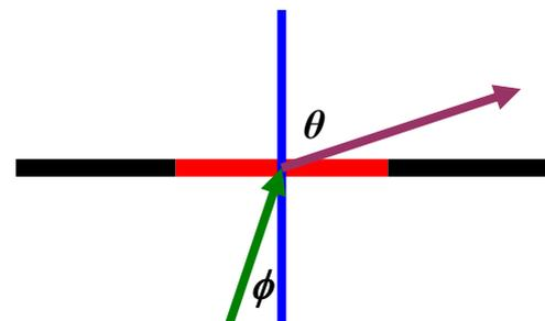
**Figure 1.** Sound incident at an angle of  $\phi$  to the normal to a panel or opening and radiated at an angle of  $\theta$  to the normal.
