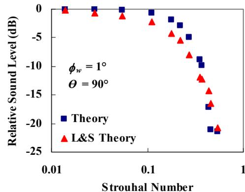
**Figure 25.** The sound level at 90° relative to that at 0° as a function of Strouhal number for an un baffled duct end opening.
