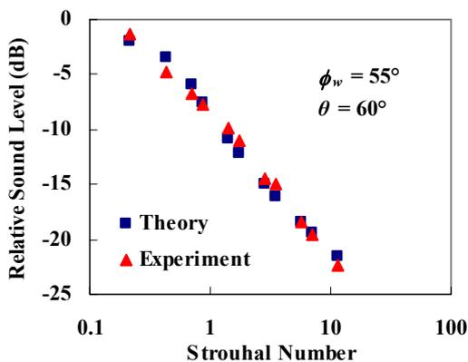
**Figure 20.** The sound level at 60° relative to that at 0° as a function of Strouhal number for an unbaffled duct end opening.
