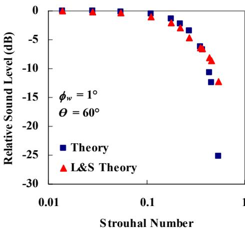
**Figure 24.** The sound level at 60° relative to that at 0° as a function of Strouhal number for an un baffled duct end opening.
