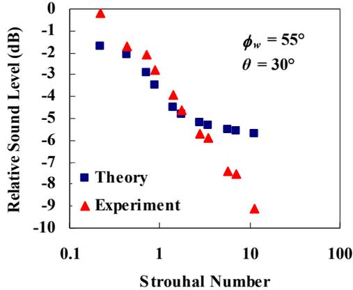
**Figure 18.** The sound level at 30° relative to that at 0° as a function of Strouhal number for an unbaffled duct end opening.
