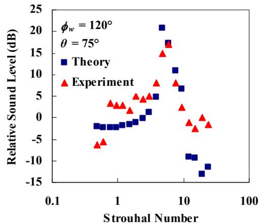
Figure 6. The sound level at 75° relative to that at 0° as a function of Strouhal number for 3 mm thick glass installed in the wall of a box.
