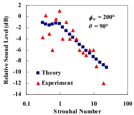
**Figure 16.** The sound level at 90° relative to that at 0° as a function of Strouhal number for an opening in the wall of a box.
