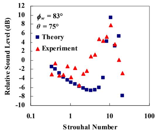
Figure 12. The sound level at  $75^\circ$  relative to that at  $0^\circ$  as a function of Strouhal number for 6 mm thick glass installed in the wall of a room.
