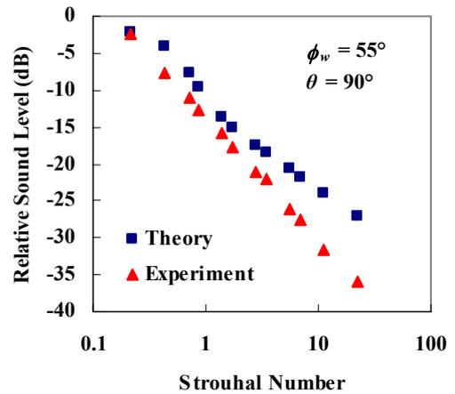
**Figure 21.** The sound level at 90° relative to that at 0° as a function of Strouhal number for an unbaffled duct end opening with a weighting angle of 55°.
