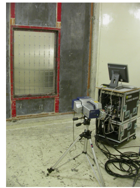
Figure 4: Picture inside the source room of the transmission loss test facility, showing the laser vibrometer.
