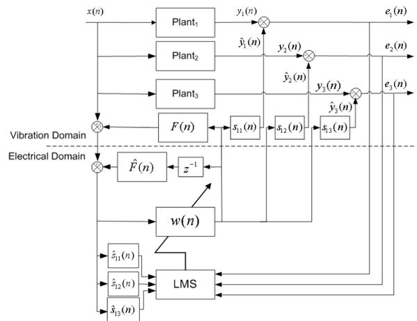
Figure 3: Detailed diagram of the [1x1x3] MISO system showing the electronic part and the vibration/acoustic part
