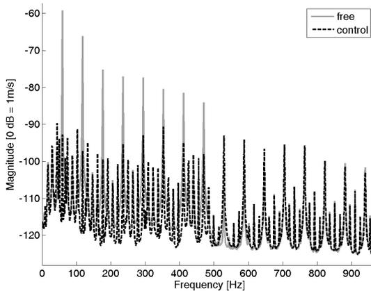
Figure 4: Velocity average spectrum of the shell scanned area with and without control.
