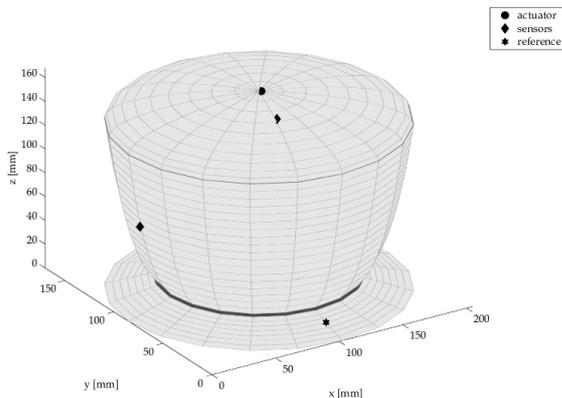
Figure 2: Simplified diagram of the structure showing the position of the error sensors, the reference sensor and the actuator
