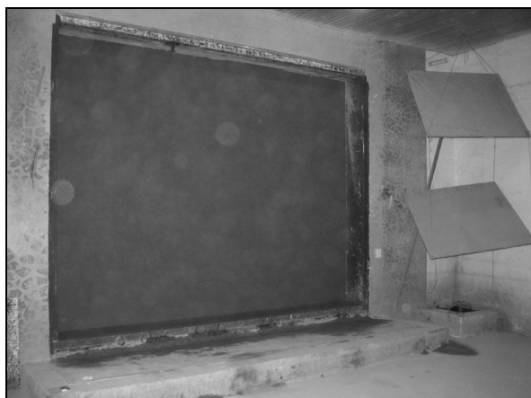
Figure 1. Test Wall and Receiver Room Diffusers.
