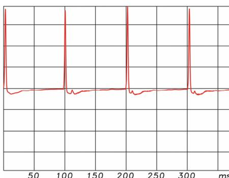
**Figure 10.** Top: Force spectra of the tapping machine, the modified tapping machine and a rubber ball according to ISO DIS 140-11. Bottom: Force-time signal of the tapping machine.
