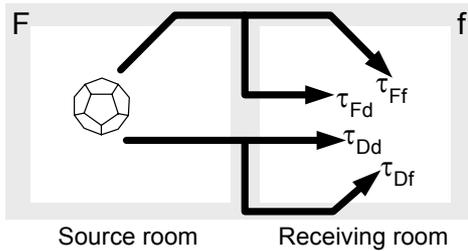
**Figure 2.** Room to room situation with sound transmission over various paths denoted by indices with capital letters for the building element in the source room (Direct or Flanking) and with lower case letters for the building element in the receiving room (direct or flanking).
