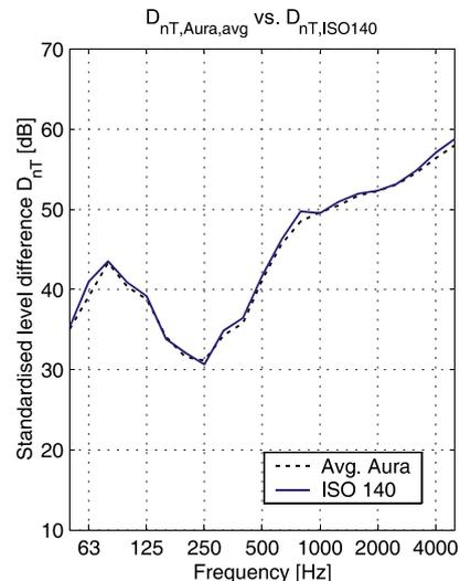
**Figure 5.** Standardized sound level difference of auralization and measurement.
