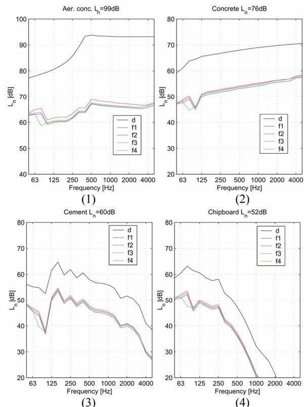
**Figure 9.** Normalised impact sound pressure levels modelled according to EN 12354, (1) to (4): bare aerated concrete, bare concrete, concrete floating floor, wooden floating floor.
