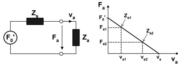
**Figure 13.** The source can be characterised through  $F_0'$  and  $Z_s$  by two measurements of force and velocity
