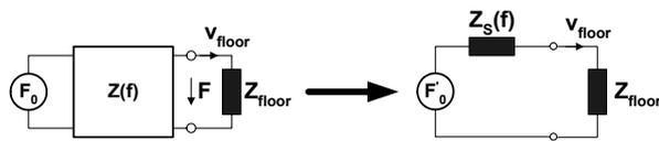
**Figure 12.** Model of a walker as a two-port, connected to the floor and its simplification
