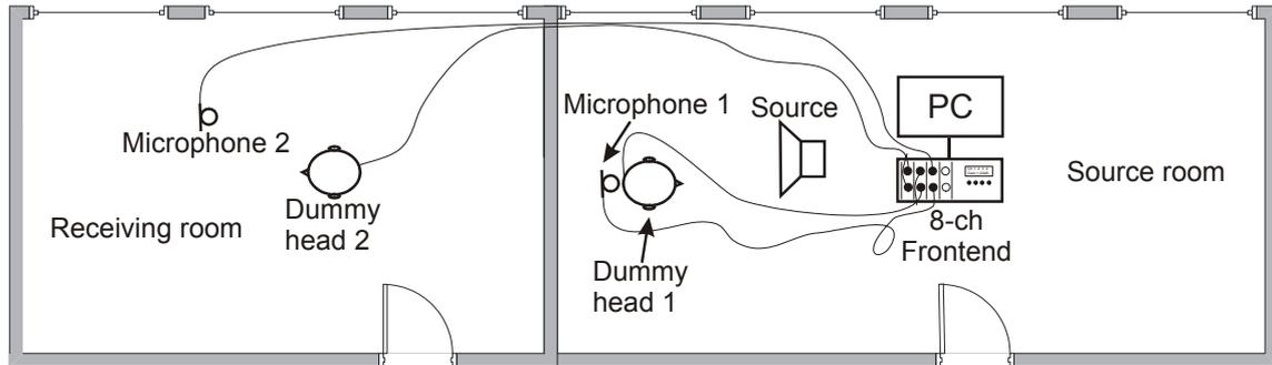
**Figure 3.** Verification test: measurement and auralization.
