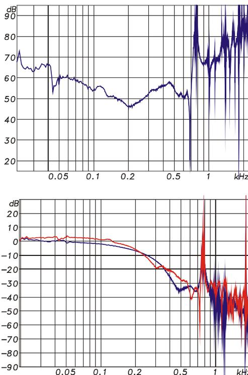
**Figure 14.** Measurement of the modified tapping machine. top: source impedance, bottom: the open-circuit force calculated twice from both forces over the load impedances. (should ideally be identical)
