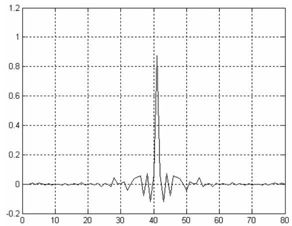
Figure 3. Loudspeaker Equaliser FIR Filter Impulse Response,  $N = 81$
