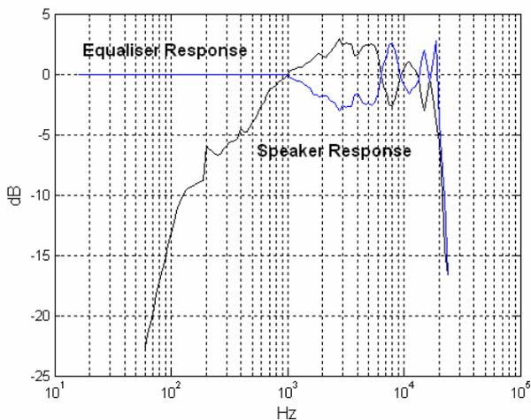
Figure 1. Loudspeaker and Corresponding Required Equaliser Responses
