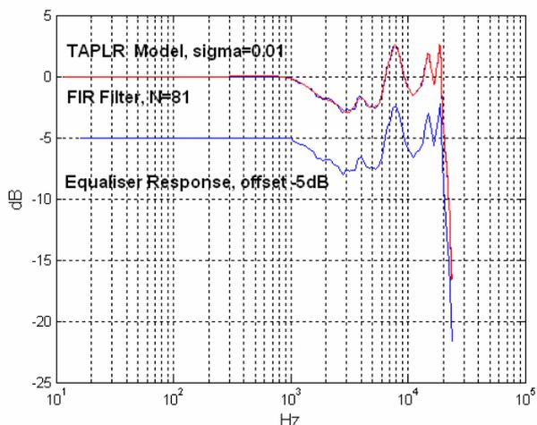
Figure 2. Loudspeaker Equaliser FIR Filter Design,  $N = 81$
