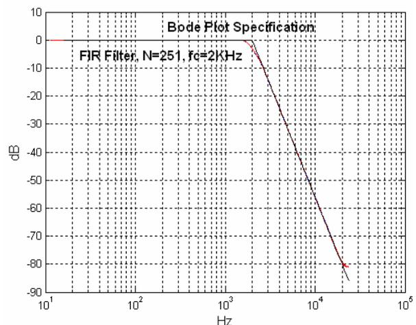
Figure 4. Lowpass FIR Filter Design,  $N = 251$
