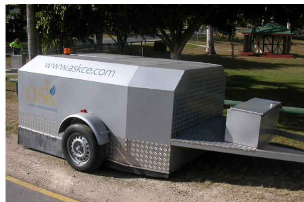
Figure 2. ‘Road Ear’ Test Rig – for CPX Testing.
