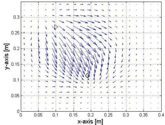
**Figure 3.** Vibration intensity plot for the controlled plate. Direction of vibration intensity at the actuator location (shown as circle) is -78.5 degrees.
