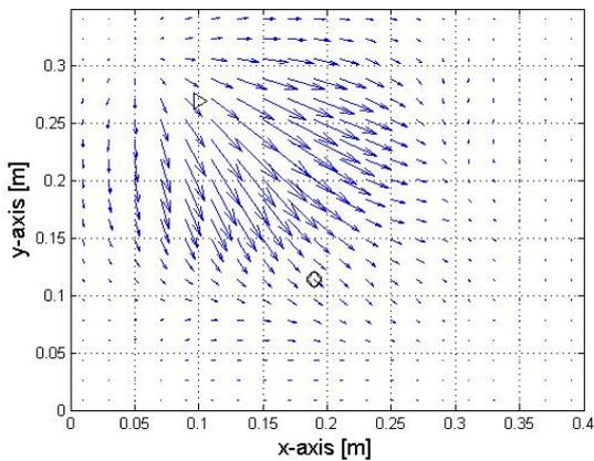
**Figure 2.** Vibration intensity plots of the panel excited by the disturbance point force at the natural frequency of mode (1,1) at 99.3 Hz. The disturbance and control source locations are denoted by the triangle and the circle respectively.
