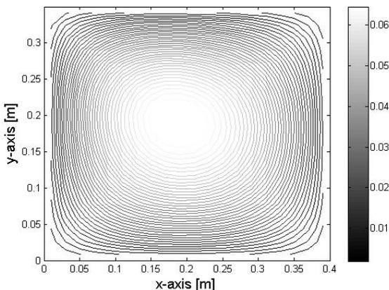
**Figure 6.** Vibration amplitude (contour) for the controlled plate. The vibration intensity direction is 90 degrees.
