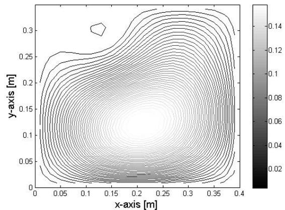
**Figure 8.** Vibration amplitude (contour) for the controlled plate using two actuators.
