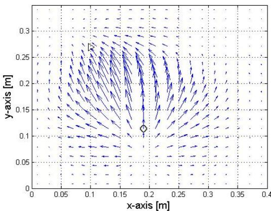
**Figure 5.** Vibration intensity plot for the controlled plate. The direction of vibration intensity at the actuator location (shown as circle) is 90 degrees.
