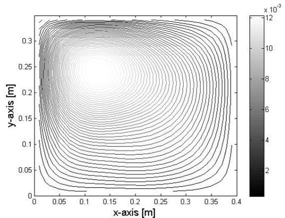
**Figure 4.** Vibration amplitude (contour) of the controlled plate. Vibration intensity direction is -78.5 degrees.
