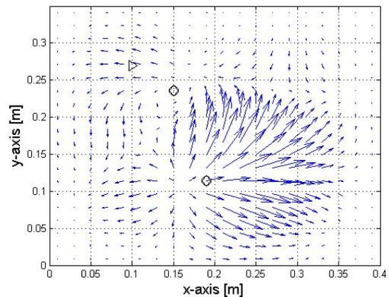
**Figure 7.** Vibration intensity plot for the controlled plate using two actuators. The locations of 2 actuators are shown as circles.
