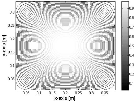
**Figure 1.** Vibration amplitude (contour) of the panel excited by the disturbance point force at the natural frequency of mode (1,1) at 99.3 Hz.
