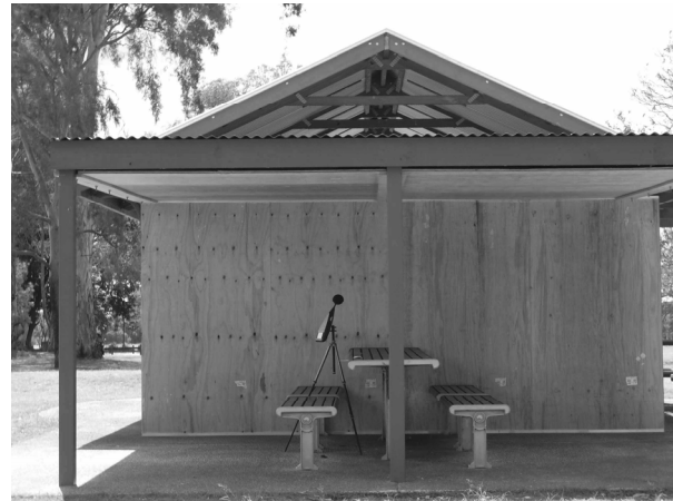
Figure 4 One-sided Enclosure with Reflective Ceiling
