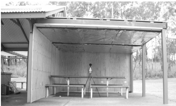
Figure 3 Two-sided Enclosure with Absorptive Ceiling
