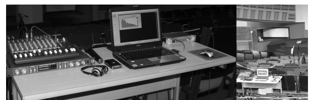
Figure 17. Acoustic measurements instrumentation in the middle of the auditorium
