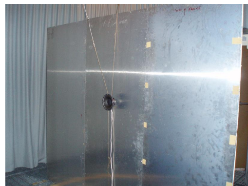
Figure 5. Experimental set-up in an anechoic room with a dipole source (vertical dipole) in front of the reflecting panels.
