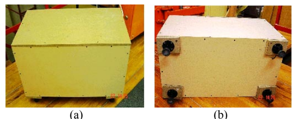
Figure 4: Views of the ‘radiation box’ (a) top surface of Armour HDF, (b) the resilient mounting feet.
