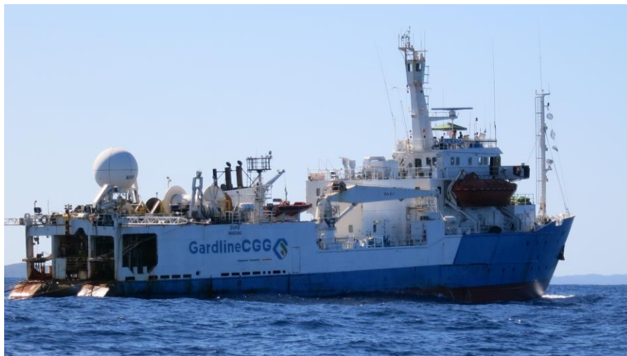
Figure 3. RV The Duke , the source vessel used in the last air gun experiment. The vessel conducted northward transects during the trials, but these were approximately 8km offshore, further out to sea than the path used by the smaller source vessel with the single air gun used in 2010 and shown in Figure 2. To improve manoeuvrability, The Duke did not deploy its long 'streamers' of hydrophones during the experiment.
