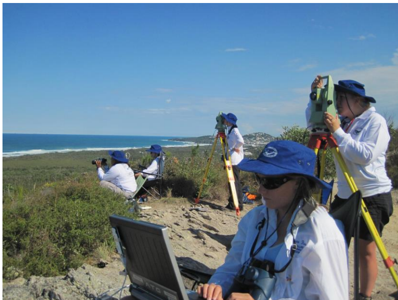
Figure 4. Observers on Emu Mt (73m), the southern observer station at Peregrine Beach. Each focal group of whales was followed by a dedicated team of observers. Horizontal and vertical bearings from the theodolites were exported directly to notebook computers running Cyclopes or VADAR software (E. Kniest, Univ. Newcastle) which calculated the position of the group in real time annotated with behaviour. Positions and behaviours were transferred in real time to the base station via the internet. This enabled the trial director at the base station to know, in real time, the positions and behaviours of all focal groups, the small vessels and the source vessel as well as the location (from the acoustic array) of vocalising animals.
