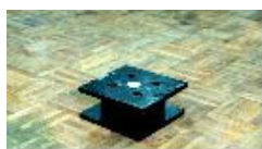
Figure 2. Photo of an individual lead core rubber bearing
