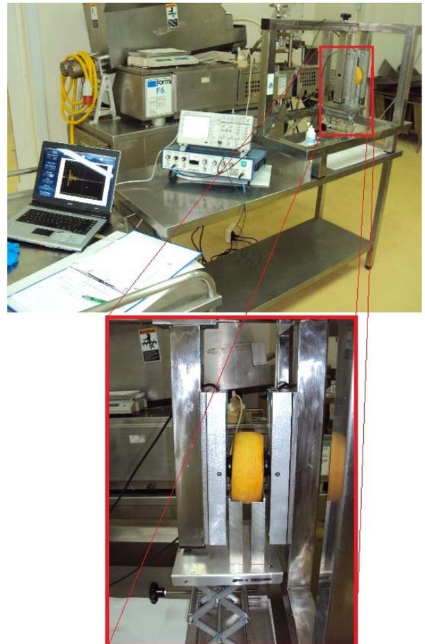
**Figure 4.** Experimental set-up for the contact measurements. Detail of the contact of the transducers with the *Torta del Casar* cheese
