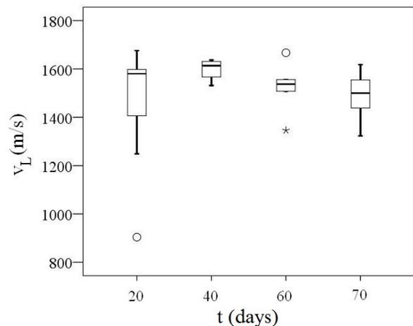
**Figure 13.** Box-and-whisker diagrams of the temporal evolution of the longitudinal wave propagation velocity,  $v_L$ , in the 32 cheeses inspected at various stages of ripening.  $\circ$ : outliers. \*: extreme cases
