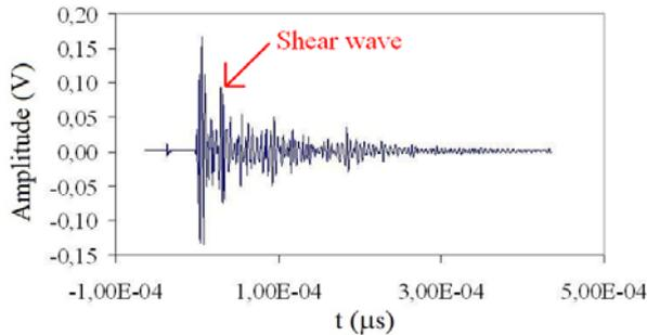
**Figure 11.** Characteristic A-scan of the same sample as in Fig. 10, but with the V150 transducer. Shown in red is the arrival of the shear wave train
