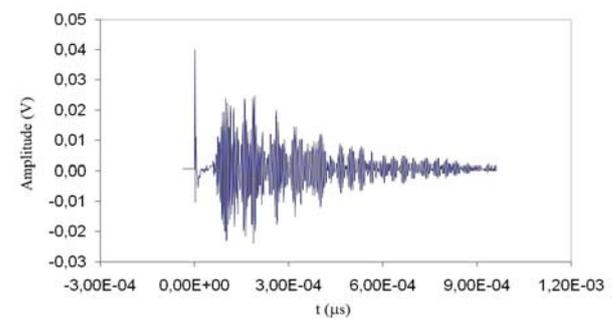
**Figure 10.** Characteristic A-scan of one of the samples inspected with the B0,05U transducer
