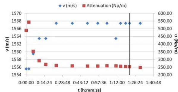
**Figure 8.** Temporal evolution of the velocity  $v$  (m/s) and attenuation  $\alpha$  (Np/m) of ultrasound waves during the coagulation process. The black vertical line indicates the optimal cutting time indicated by the master cheese-maker
