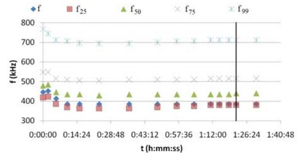
**Figure 9.** Temporal evolution of the central frequency and cumulative frequencies at 25% ( $f_{25}$ ), 50% ( $f_{50}$ ), 75% ( $f_{75}$ ), and 99% ( $f_{99}$ ) of the FFT of ultrasound signals obtained during the coagulation process. The black vertical line indicates the optimal cutting time indicated by the master cheese-maker
