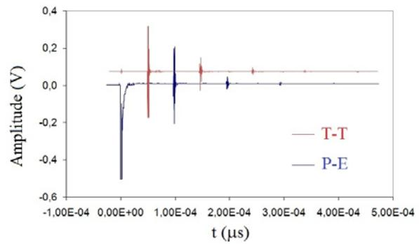
**Figure 6.** Comparison of the A-scans obtained with the V314 transducer in through-transmission (TT) and pulse-echo (PE) modes for a distance between transducers of  $d=7.21$  cm
