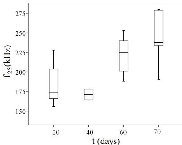
**Figure 15.** Box-and-whisker diagrams of the temporal evolution of the 25% cumulative frequency ( $f_{25}$ ) of the FFT obtained with the V1548 pair of transducers in the ultrasonic inspection of the 32 cheeses, at different stages of ripening
