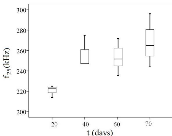
**Figure 16.** Box-and-whisker diagrams of the temporal evolution of the 25% cumulative frequency ( $f_{25}$ ) of the FFT obtained with the V150 pair of transducers in the ultrasonic inspection of the 32 cheeses, at different stages of ripening
