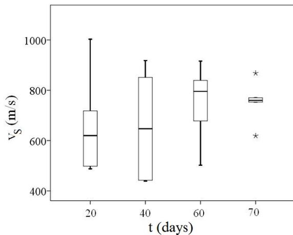
**Figure 14.** Box-and-whisker diagrams of the temporal evolution of the shear wave propagation velocity,  $v_s$ , in the 32 cheeses inspected at various stages of ripening.  $\circ$ : outliers.  $*$ : extreme cases
