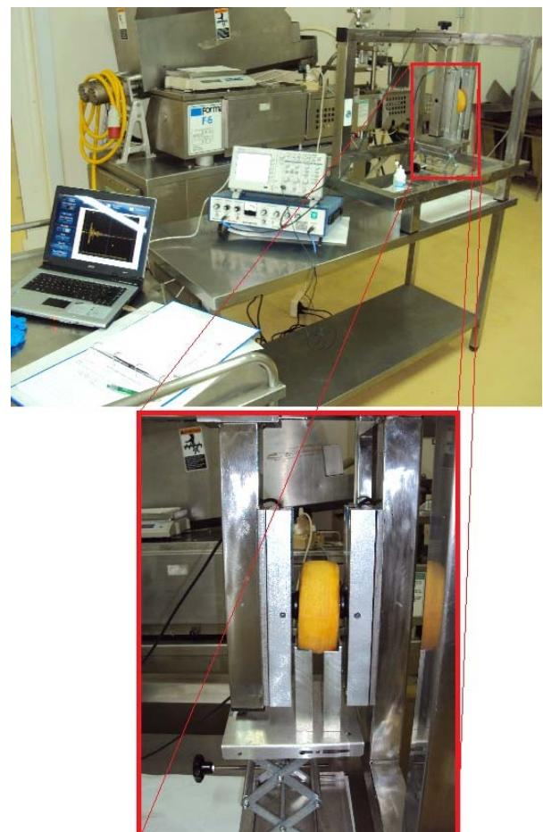
**Figure 4.** Experimental set-up for the contact measurements. Detail of the contact of the transducers with the *Torta del Casar* cheese
