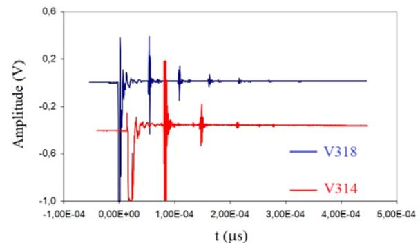
**Figure 7.** Comparative study of the A-scans obtained with the V318 and V314 transducers
