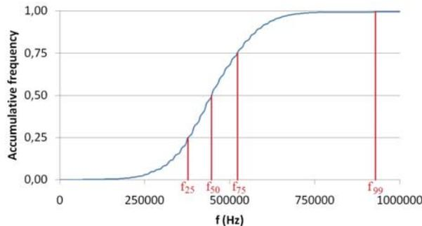
**Figure 3.** Example of an integrated periodogram of the signal received by the Panametrics V318 transducer. In red are marked the cumulative frequency values at 25% ( $f_{25}$ ), 50% ( $f_{50}$ ), 75% ( $f_{75}$ ), and 99% ( $f_{99}$ ) of the FFT
