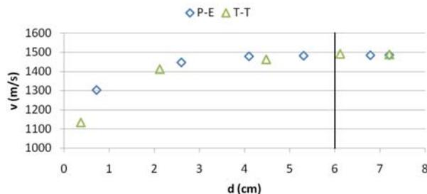
**Figure 5.** Study with the V314 transducer of the evolution of the speed of ultrasound  $v$  versus distance  $d$  travelled by the ultrasound beam in pulse-echo and through-transmission modes. The vertical line indicates the transducer's near-field length
