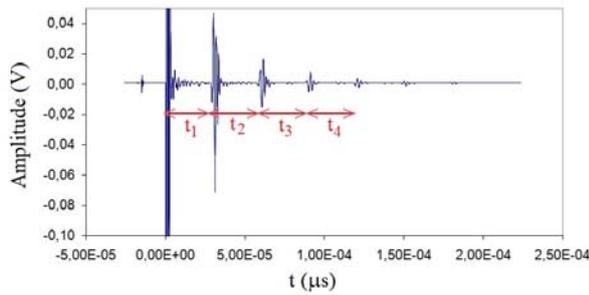
**Figure 2.** Example of the A-scan signal received by the Panametrics V314 transducer. After the trigger pulse, one observes the echoes of the ultrasound signal
