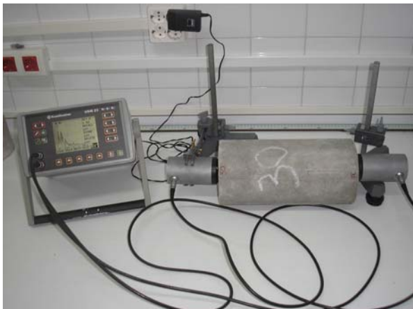
Figure 1. Ultrasonic device for velocity measurements
