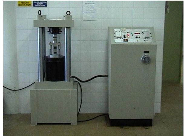
Figure 4. Hydraulic press for compressive strength S_C measurements
