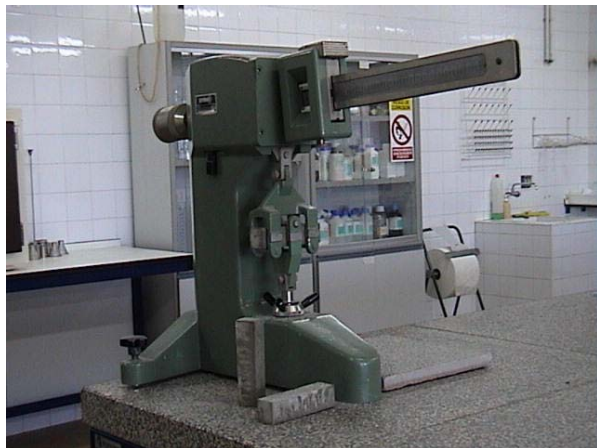
Figure 3. Device for flexion strength S_F measurements
