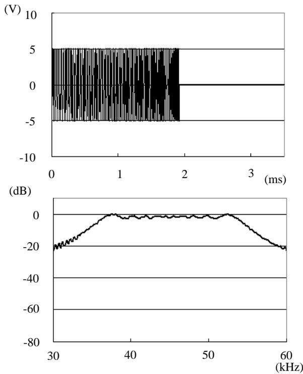
Figure 3. Waveform and spectrum of the Chirp wave
