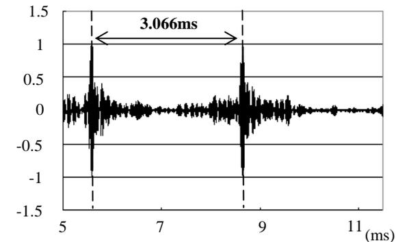
Figure 11. Example of compressed result of the received signal when  $v=1.7$  m/s
