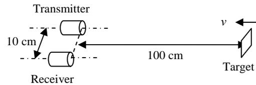
Figure 2. Arrangement of transducers and moving target for speed measurement
