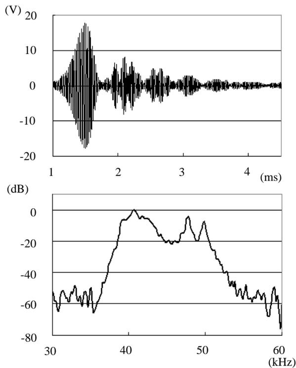
Figure 4. Reference received signal of the Chirp wave
