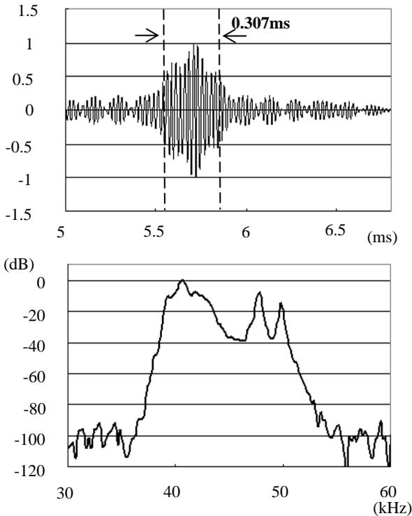
Figure 7. Example of compressed pulse of the Chirp wave
