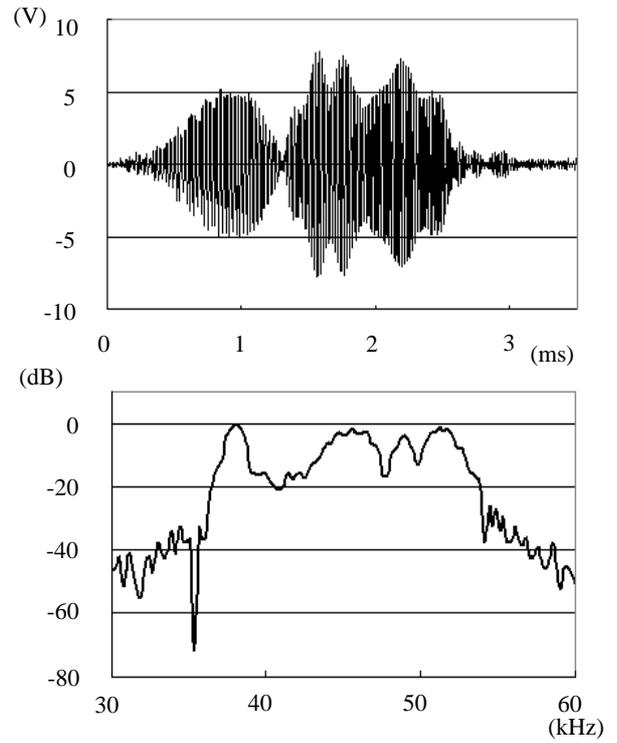
Figure 5. Waveform and spectrum of the SCT signal
