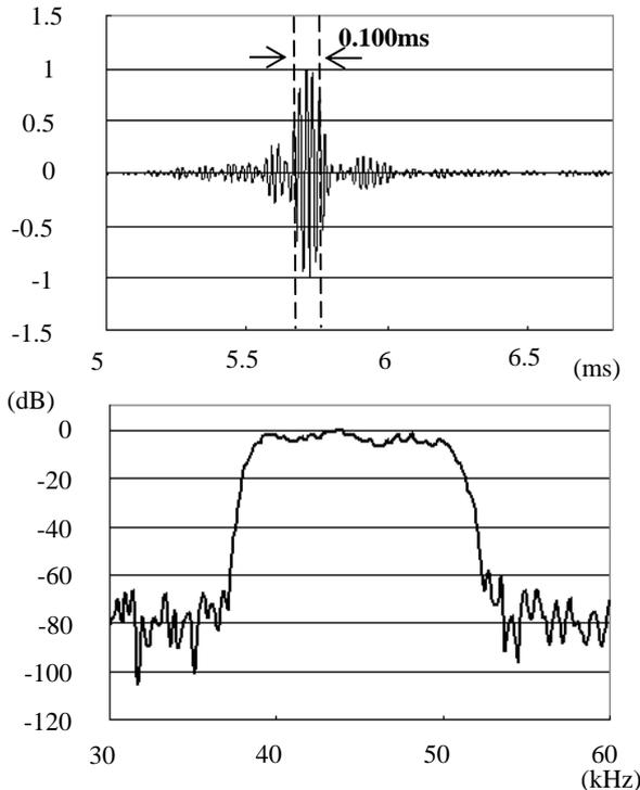
Figure 8. Example of compressed pulse of the SCT signal
