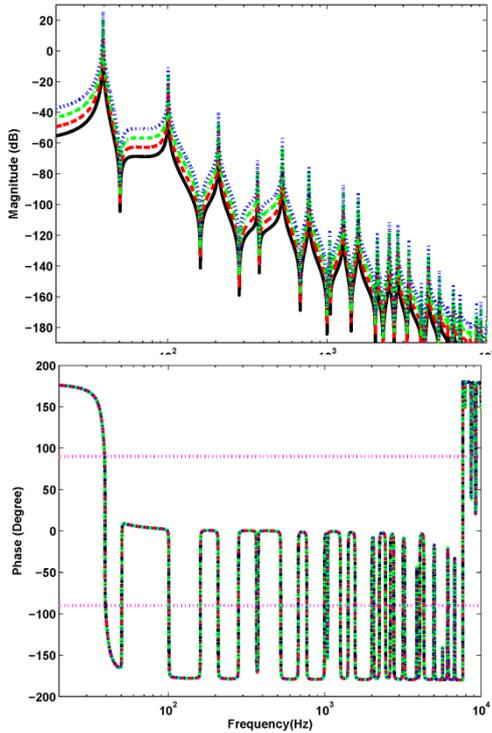
**Figure 5.** The effect of magnitude as the 1<sup>st</sup> mode controller gain change of open loop transfer function of the clamped beam at 0.7L which is excited by a force at 0.2L, and set the 1<sup>st</sup> mode controller damping ratio,  $5 \times 10^{-5}$ , gain,  $5 \times 10^{-5}$  (solid line),  $1 \times 10^{-4}$  (dashed line),  $2 \times 10^{-4}$  (dash-dotted) and  $4 \times 10^{-4}$  (dotted line).
