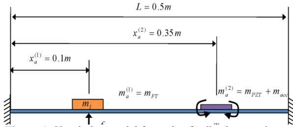
**Figure 1.** Simulation model for active feedback control system for a clamped beam with a sensor/actuator pair system.
