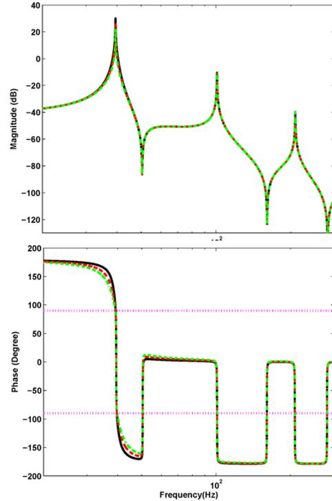
**Figure 4.** The effect of magnitude as the 1<sup>st</sup> mode controller damping ratio change of open loop transfer function of the clamped beam at  $0.7L$  which is excited by a force at  $0.2L$ , and set the 1<sup>st</sup> mode controller gain,  $4 \times 10^{-4}$ , damping ratio,  $3 \times 10^{-2}$  (solid line),  $5 \times 10^{-2}$  (dashed line) and  $7 \times 10^{-2}$  (dash-dotted line).
