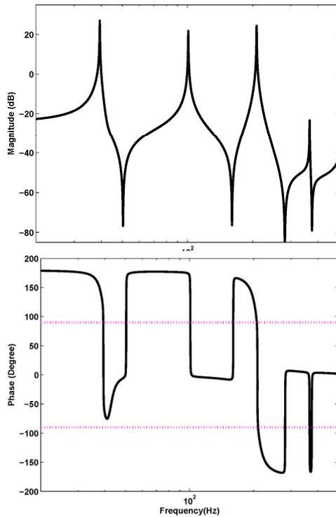
**Figure 8.** The final tuned open loop transfer function response of the clamped beam at  $0.7L$  which is excited by a force at  $0.2L$ , and set the 1<sup>st</sup> mode controller gain,  $4 \times 10^{-4}$ , 3<sup>rd</sup> mode controller gain,  $2 \times 10^{-5}$  and all controller damping ratios are  $5 \times 10^{-2}$ .
