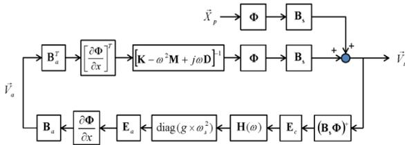
**Figure 3.** Block diagram for active vibration control using PPF controllers.
