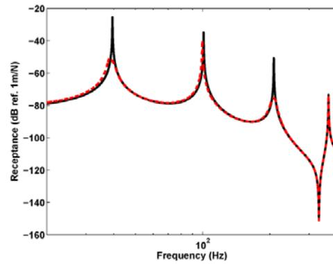
**Figure 9.** SISO PPF control performance of the clamped beam excited by the moment pair at  $0.7L$ , and uncontrolled response (solid line) and controlled response (dashed line).
