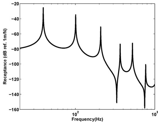
Figure 2. The calculated receptance of the beam at  $0.7L$  of mass-loaded beam which is excited by a force at  $0.2L$ .
