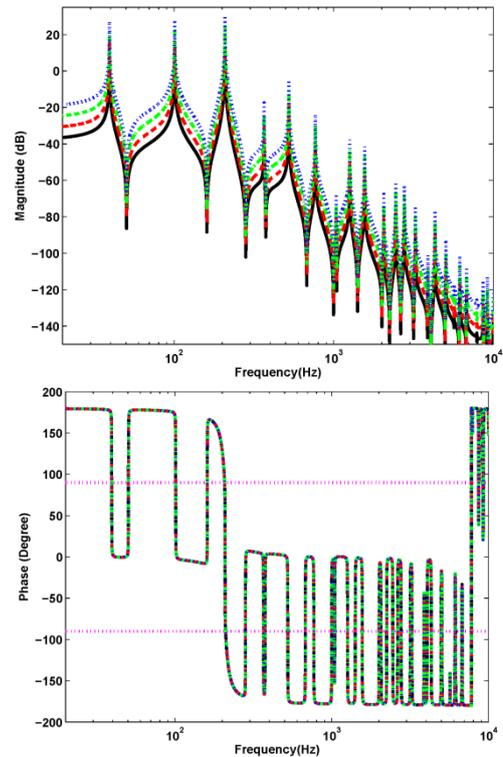
**Figure 7.** The effect of magnitude as the 3<sup>rd</sup> mode controller gain change of open loop transfer function of the clamped beam at 0.7L which is excited by a force at 0.2L, and set the 3<sup>rd</sup> mode controller damping ratio,  $5 \times 10^{-2}$ , gain,  $5 \times 10^{-6}$  (solid line),  $1 \times 10^{-5}$  (dashed line),  $2 \times 10^{-5}$  (dash-dotted) and  $4 \times 10^{-5}$  (dotted line).
