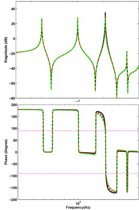
**Figure 6.** The effect of magnitude as the 3<sup>rd</sup> mode controller damping ratio change of open loop transfer function of the clamped beam at 0.7L which is excited by a force at 0.2L, and set the 3<sup>rd</sup> mode controller, gain,  $4 \times 10^{-5}$ , damping ratio,  $3 \times 10^{-2}$  (solid line),  $5 \times 10^{-2}$  (dashed line) and  $7 \times 10^{-2}$  (dash-dotted line).
