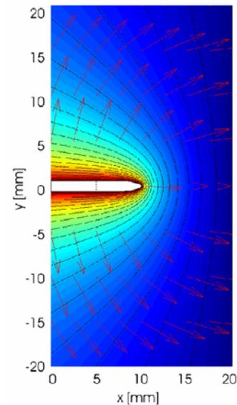
**Figure 3.** The electric field distribution between the needle and the infinite plate electrode on the right side of the picture. Arrows represent electric field lines.
