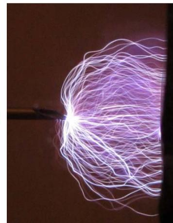
**Figure 4.** Discharge at 1-needle to 2-electrically separated plate electrode arrangement.
