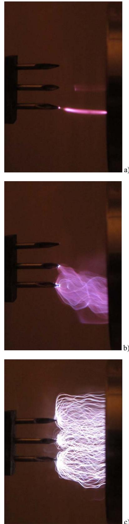
**Figure 2.** Photographs of 3-needle-to-plate electrical discharge regimes formed in the resonator by increasing the sound pressure level with a frequency of 500 Hz and constant DC voltage  $U_s = -25 \text{ kV}$ ; a)  $P=0 \text{ Pa}$ ,  $U_D = -2 \text{ kV}$ ; b)  $P=1210 \text{ Pa}$ ,  $U_D = -4 \text{ kV}$ ; c)  $P=5380 \text{ Pa}$ ,  $U_D = -7.2 \text{ kV}$ . Exposure time is 1/30 s.
