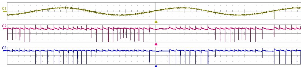
**Figure 5.** The time course of acoustic pressure amplitude at the reflector surface C1, and the current waveforms through either part (separated at nod pressure plane) of plate electrode: C2 - closer to the reflector, C3 - further-out from the reflector.
