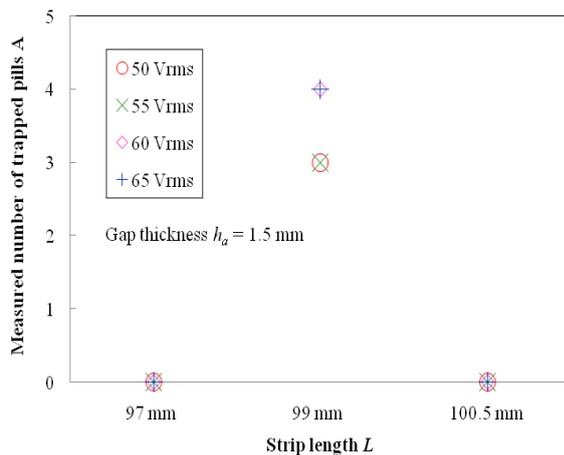
Figure 6. Measured number of trapped pills A for different strip lengths at resonance for different input voltages.
