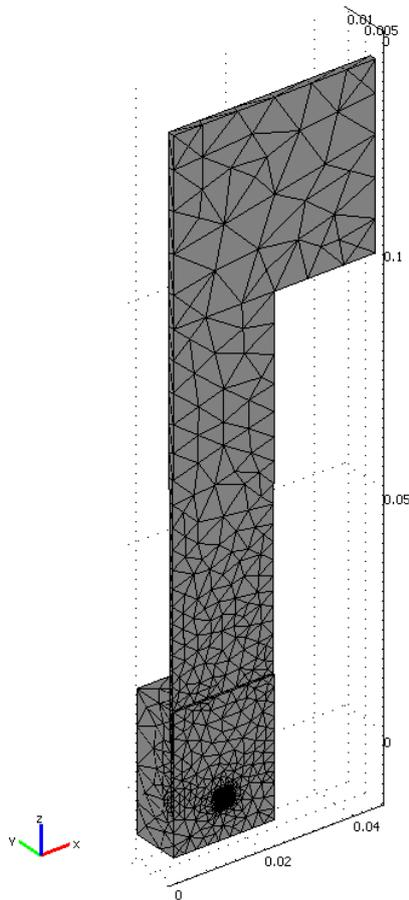
Figure 2. 3D FEM analyses of the half structure in air when vibration displacement amplitude (0-peak) of upper part of metal plate is 10 μm.
