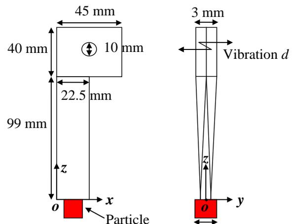
**Figure 1.** Structure and size of the W-shaped ultrasonic actuator with two V-shaped metal strips.
