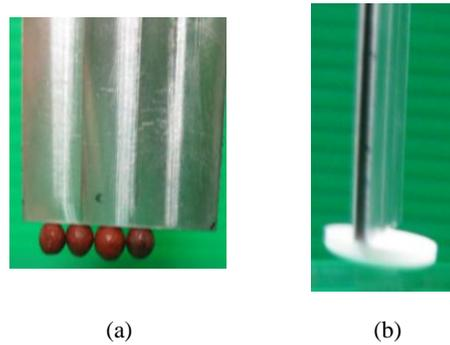
Figure.3 Trapping of medicine pills in air by the actuator
