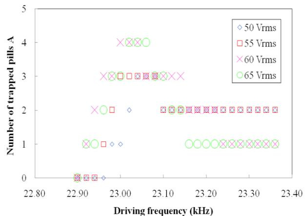
Figure 4. Experimental relationship between the number of trapped pills A and the driving frequency in air under different input voltages.
