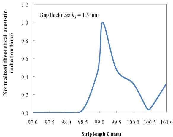
Figure 5. Calculated relationship between the normalized trapping force acting on pill A and the strip length.
