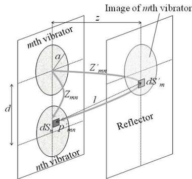
Figure 2: Equivalent model for calculation.
