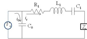
Figure 3: Equivalent circuit with acoustic radiation impedance.
