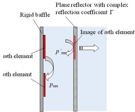
Figure 1: Geometry model of transducer array with a reflector.
