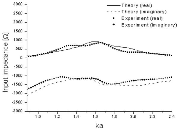
Figure 9: Input impedance of the 13th vibrator in the  $5 \times 5$  transducer array with one driving vibrator.
