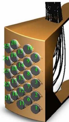
Figure 8: Structure of the  $5 \times 5$  transducer array.
