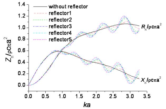
Figure 7: Normalized total radiation impedance change with  $ka$ .
