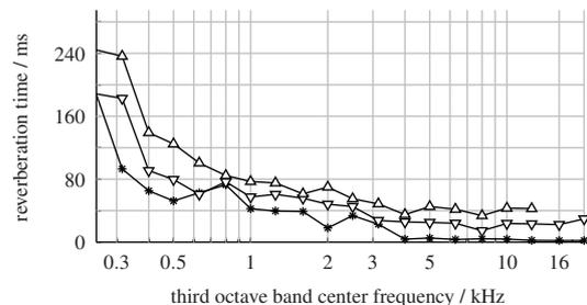
Figure 2: Reverberation time of the laboratory room where all listening experiments presented here took place. Early decay time (stars),  $T_{20}$  (downward pointing triangles), and  $T_{30}$  (upward pointing triangles).
