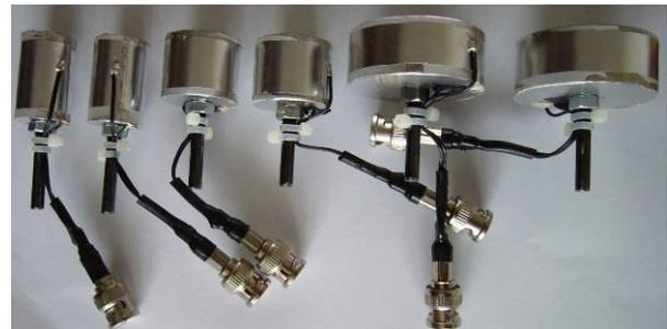
**Figure 2.** Transducers constructed using EMFi film
