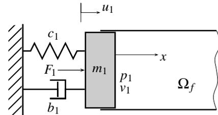
Figure 1: One-dimensional model of fluid bounded by mass-spring-damper system (MSD) as substitute for flexible wall.
