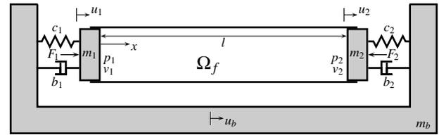
Figure 3: One-dimensional fluid with MSDs on either side and an additional mass  $m_b$ .
