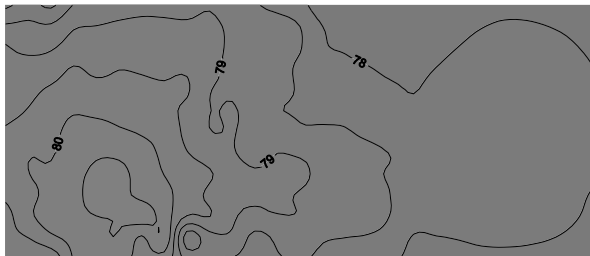
Figure 9. Distribution of the values of the A-weighted sound pressure level, in dB, in the workshop room
