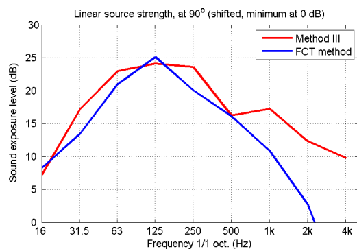
Figure 12. Linear source strength, determined according to Method III and by using a non-linear FCT method. Vertical axis has been shifted to start at 0 dB.
