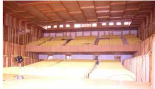
Fig.5 1/10 Scale model for experiment.
