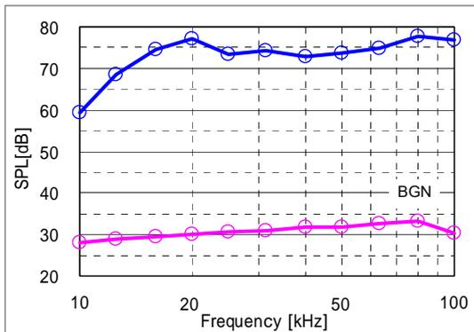
Fig.2 SPL at 15cm distance from the new dodecahedral loudspeaker.
