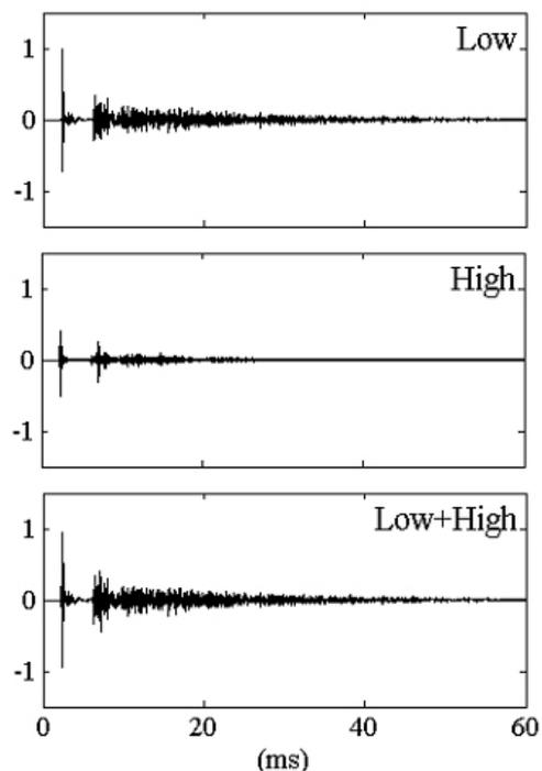
Fig.10 Room IR's measured by two miniature dodecahedral loudspeakers (Low and High), and synthesized one.
