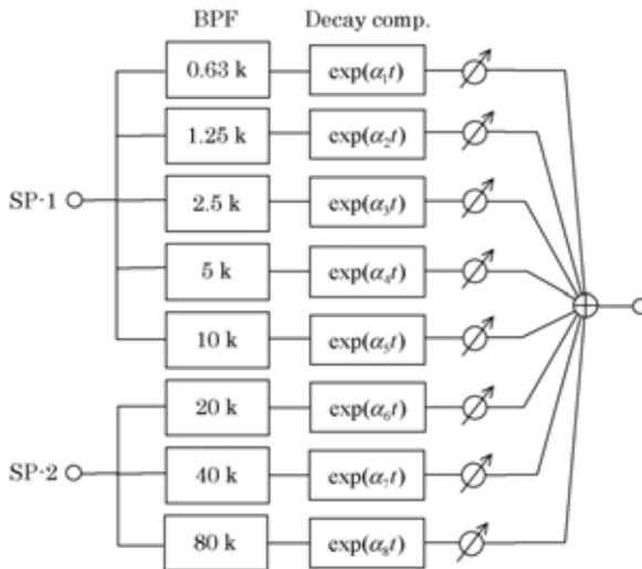
Fig.12 Block diagram of signal processing for auralization.
