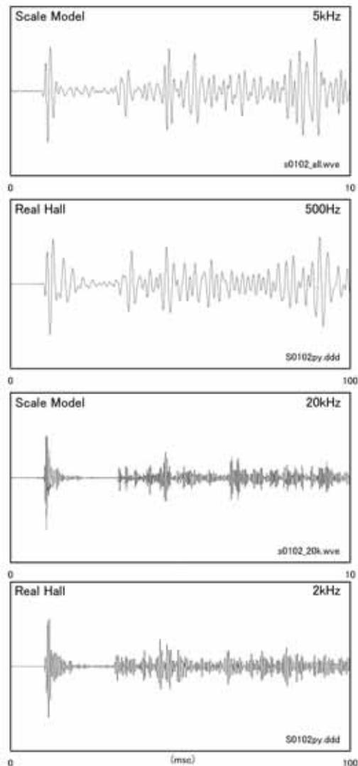
Fig.6 Comparison of reflectogram in a scale model measured with 1/8 inch microphone and in the real hall: 1/1 oct. band response at center main-floor seat.
