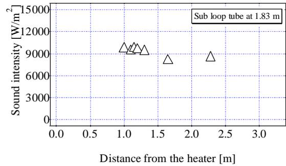
Figure 8 Sound intensity distributions with the sub-loop tube at 1.83 m from the upper end of the prime mover stack.
