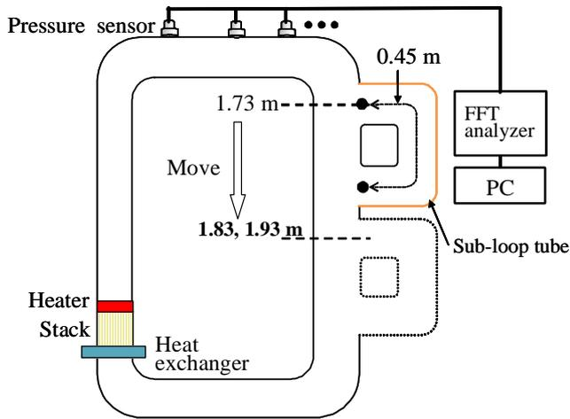
Figure 1 Experimental setup of the loop-tube-type thermoacoustic system.
