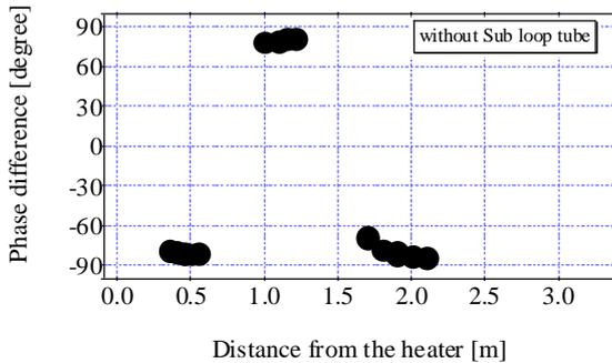
Figure 10 Distributions of the phase difference between the sound pressure and particle velocity without the sub-loop tube.
