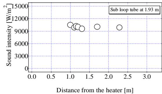
Figure 9 Sound intensity distributions with the sub-loop tube at 1.93 m from the upper end of the prime mover stack.
