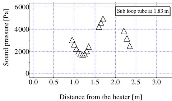
Figure 4 Sound pressure distributions with the sub-loop tube at 1.83 m from the upper end of the prime mover stack.
