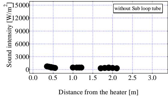
Figure 6 Sound intensity distributions without the sub-loop tube.
