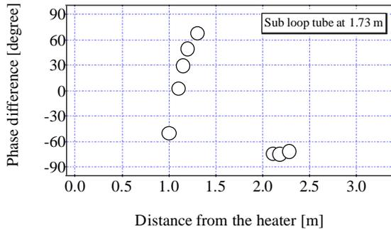
Figure 11 Distributions of phase difference between the sound pressure and particle velocity with the sub-loop tube at 1.73 m from the upper end of the prime mover stack.
