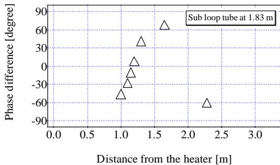
Figure 12 Distributions of phase difference between sound pressure and particle velocity with the sub-loop tube at 1.83 m the upper end of the prime mover stack.
