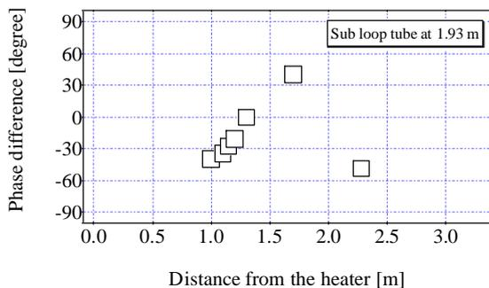
Figure 13 Distributions of phase difference between the sound pressure and particle velocity with the sub-loop tube at 1.93 m from the upper end of the prime mover stack.
