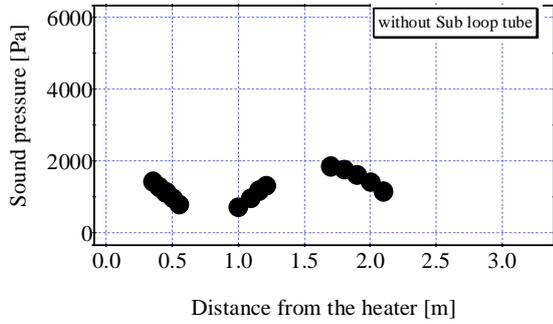
Figure 2 Sound pressure distributions without the sub-loop tube.
