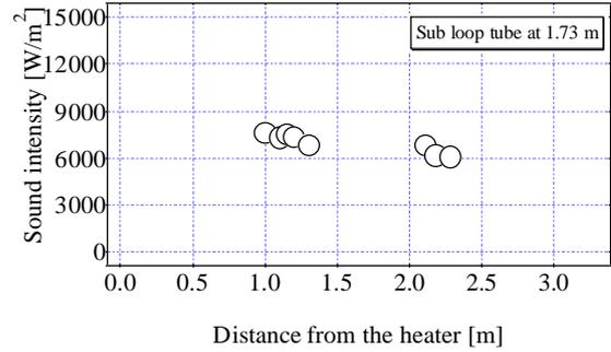
Figure 7 Sound intensity distributions with the sub-loop tube at 1.73 m from the upper end of the prime mover stack.
