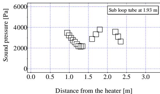
Figure 5 Sound pressure distributions with the sub-loop tube at 1.93 m from the upper end of the prime mover stack.
