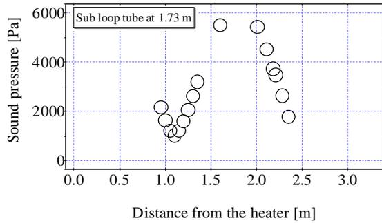
Figure 3 Sound pressure distributions with the sub-loop tube at 1.73 m from the upper end of the prime mover stack.
