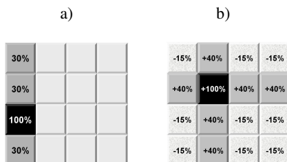
Figure 15. Distribution of voltages at A3 array transducers when activating one element in the system: a) active – single columns, or interchangeably rows are activated [12], b) passive – the whole array is activated [13].
