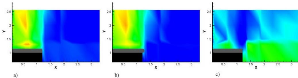
**Figure 5.** a) Rectangular edge – 2000 Hz, b) Rounded edge – 2000 Hz, c) Difference in IL between a) and b)
