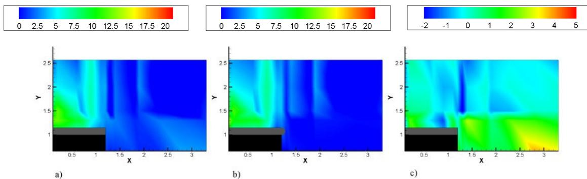
**Figure 7.** a) Rectangular edge – 8000 Hz, b) Rounded edge – 8000 Hz, c) Difference in IL between a) and b)
