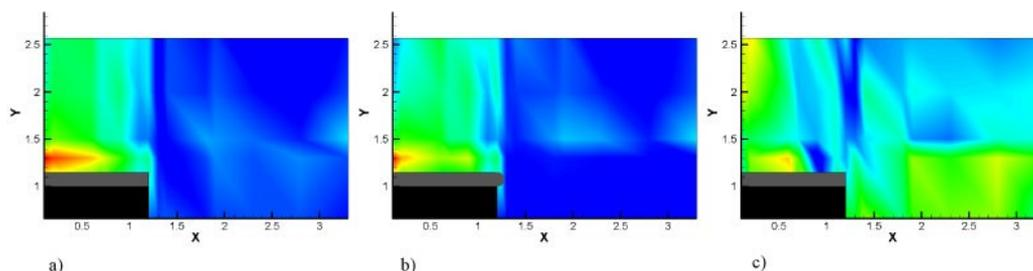
**Figure 8.** a) Rectangular edge – 10 kHz, b) Rounded edge – 10 kHz, c) Difference in IL between a) and b)
