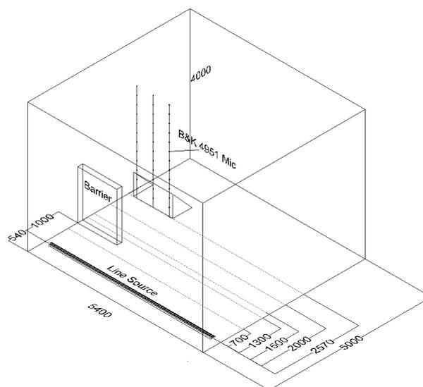
**Figure 3.** Layout of the semi-anechoic chamber and experiment setup
