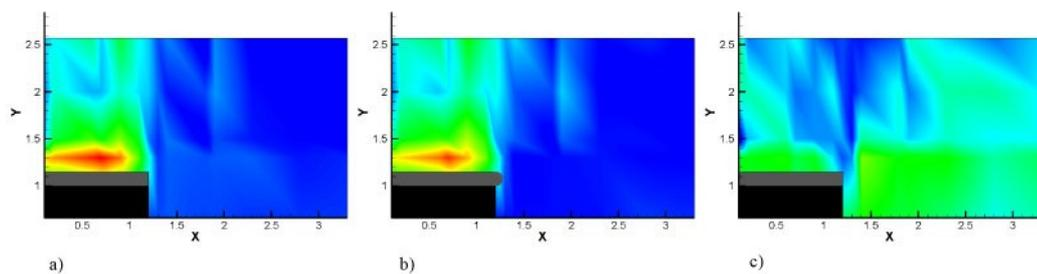
**Figure 6.** a) Rectangular edge – 4000 Hz, b) Rounded edge – 4000 Hz, c) Difference in IL between a) and b)
