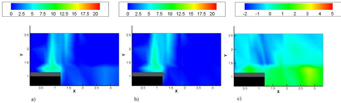
**Figure 4.** a) Rectangular edge – 500 Hz, b) Rounded edge – 500 Hz, c) Difference in IL between a) and b)
