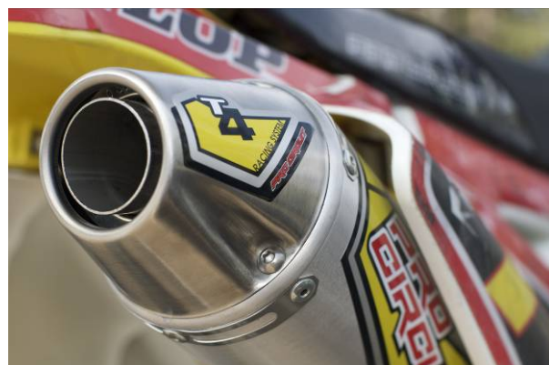
Figure 5. Detail of an aftermarket exhaust, fitted with an interchangeable tailpipe insert
