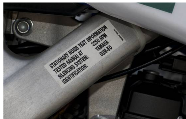
Figure 1. Detail of a noise compliance sticker affixed to motorcycle chassis
