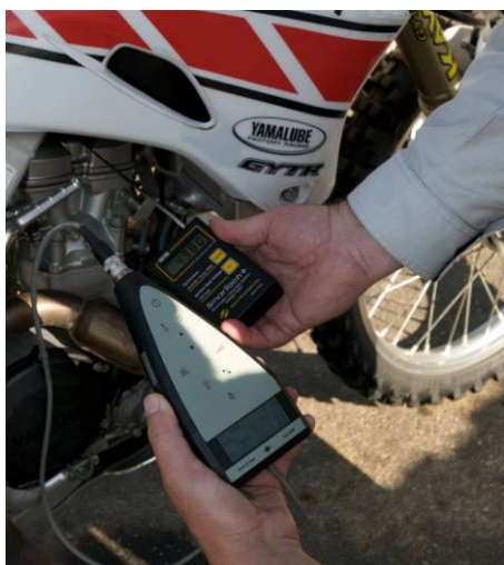
Figure 2. Simultaneous sound level meter and tachometer readings for stationary measurements
