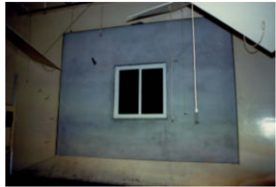
Photo 4. Window with a PVC frame and two sliding panes with a 3mm monolithic glass
