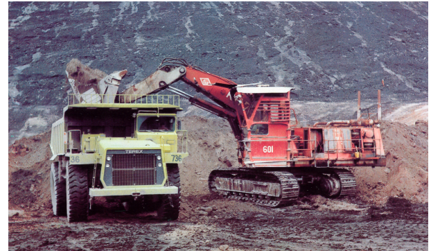
Figure 2. Hydraulic excavator loading burden into 77 tonne truck
