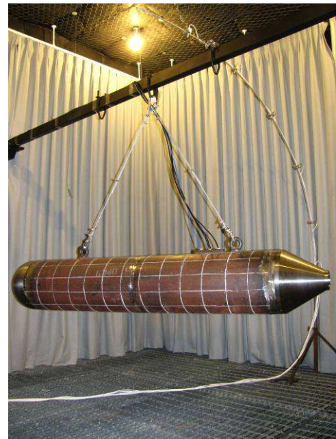
Figure 6 The actual rig of sound pressure measurement
